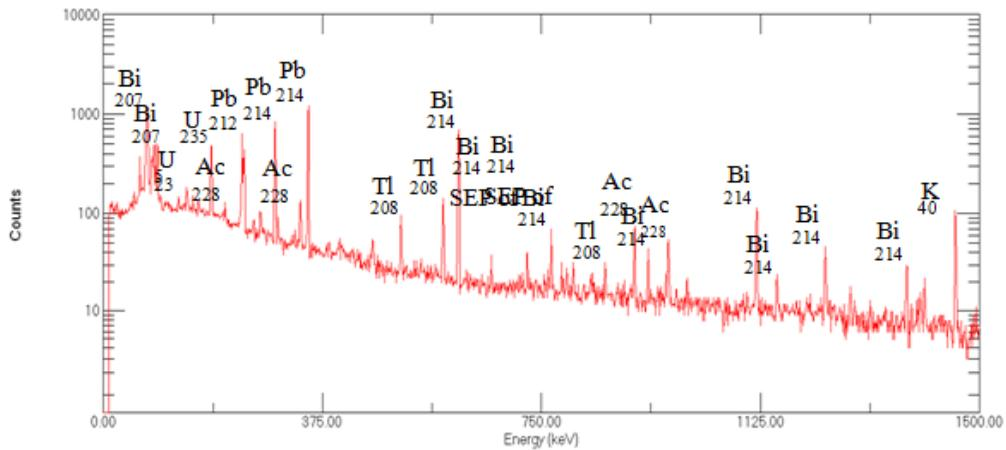
**Figure 3.2:** The energy spectrum of the Coal ash sample
