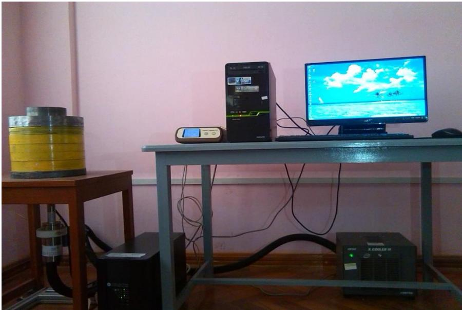
**Figure 2.2:** The photo of the experimental set up of HPGe detection system
