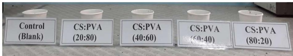
**Figure 1:** Experiment for determination of water retention of soil
