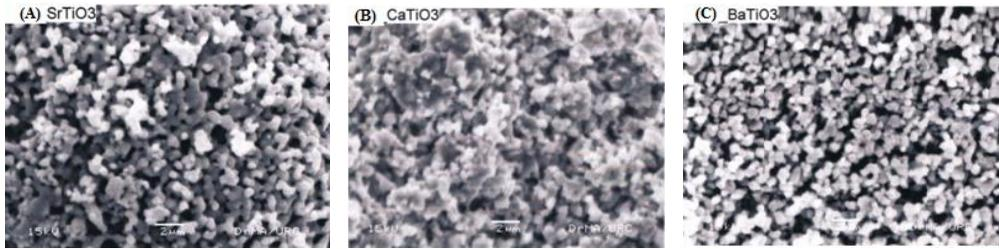
**Figure 2:**The scanning electron micrograph of (a) SrTiO<sub>3</sub>/ITO glass (b) CaTiO<sub>3</sub>/ITO glass (c) BaTiO<sub>3</sub>/ITO glass thin film.
