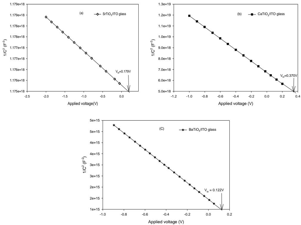
**Figure 3:**  $1/C^2 - V$  plots for Perovskite-type (a) SrTiO<sub>3</sub>/ITO glass (b) CaTiO<sub>3</sub>/ITO glass and (c) BaTiO<sub>3</sub>/ITO glass thin film.
