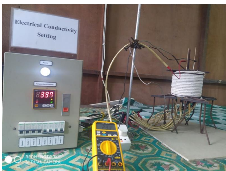
Figure 6 Experimental set-up of resistivity measurement
