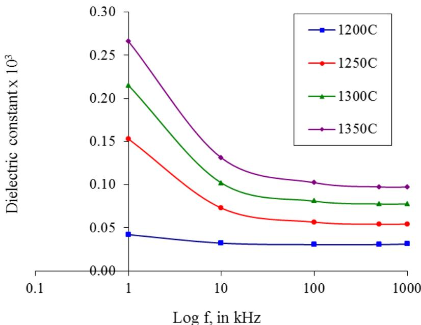
**Figure 13** The variations of dielectric constant with frequency
