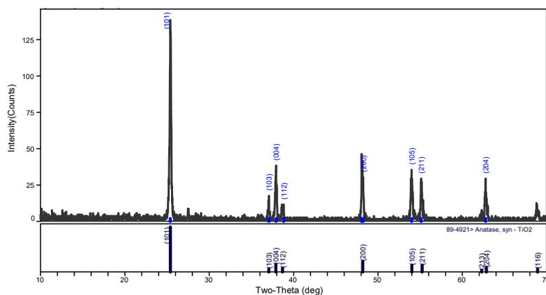
**Figure 2** XRD Spectrum of TiO<sub>2</sub>
