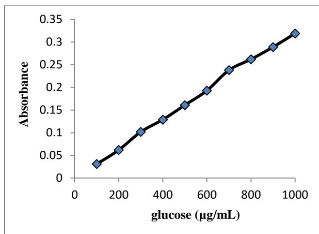
**Figure 2** Plot of absorbance as a function of weight of glucose
