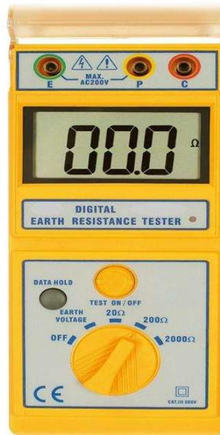
**Figure 2.1:** Earth resistance tester (Model 2720 ER)
