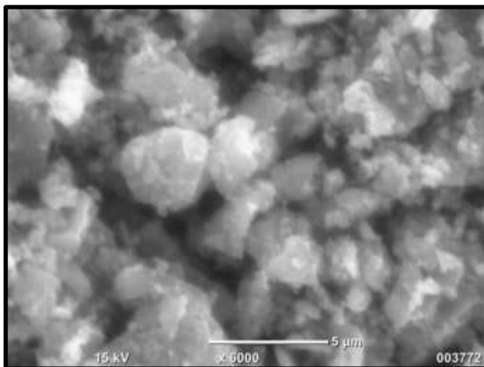
**Figure 2 (a)** The SEM micrographs of TiO<sub>2</sub> nanoparticles with NaOH (0.1 g).
