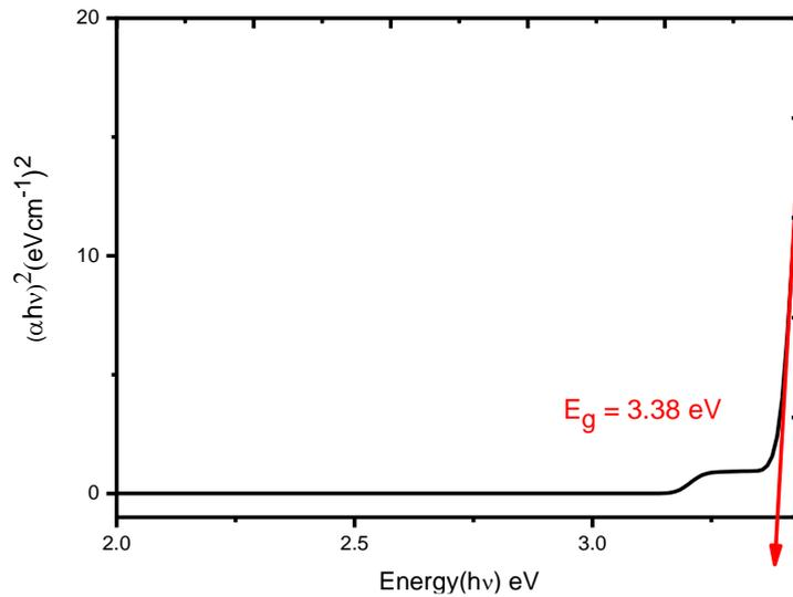
**Figure 3 (d)** The plot of extrapolation for TiO<sub>2</sub> nanoparticles from NaOH (0.5 g) with deionized water.
