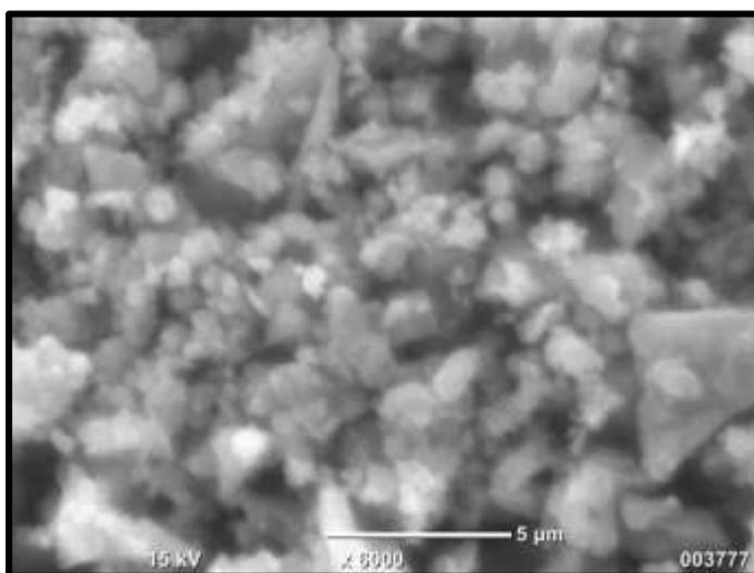
**Figure 2 (b)** The SEM micrographs of TiO<sub>2</sub> nanoparticles with NaOH (0.3 g).
