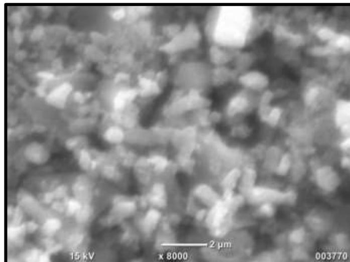
**Figure 2 (d)** The SEM micrographs of TiO<sub>2</sub> nanoparticles with NaOH (0.5 g) and deionized water.
