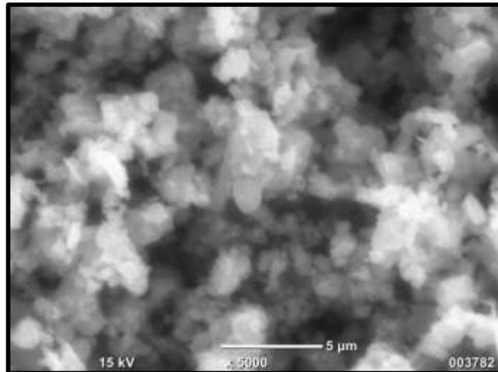
**Figure 2 (c)** The SEM micrographs of TiO<sub>2</sub> nanoparticles with NaOH (0.5 g).
