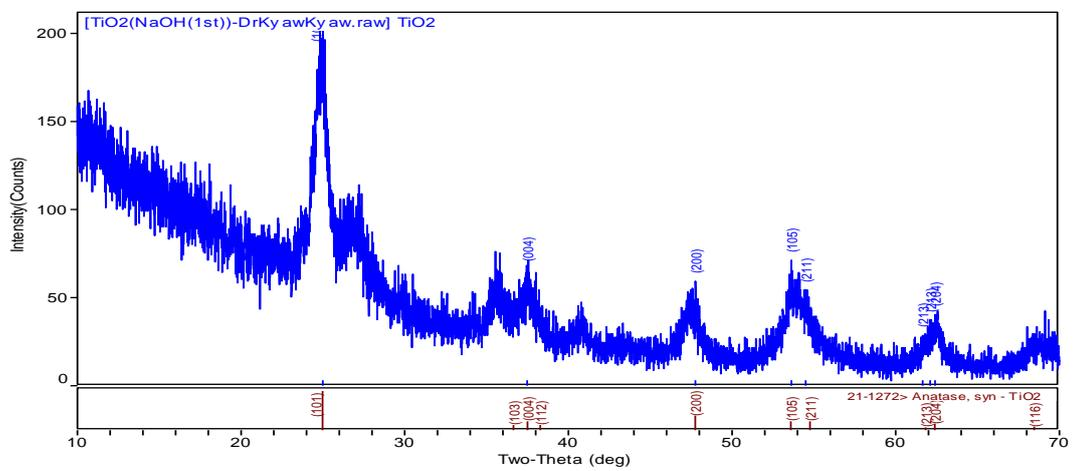
**Figure 1 (d)** XRD profiles of TiO<sub>2</sub> nanoparticles from NaOH(0.5g) with deionized water.
