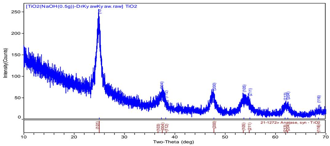
**Figure 1 (c)** XRD profiles of TiO<sub>2</sub> nanoparticles from NaOH(0.5g).
