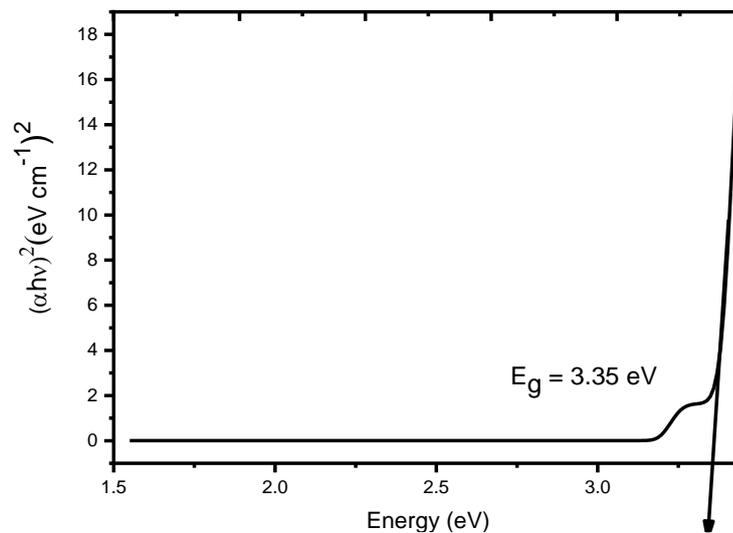
**Figure 3 (b)** The plot of extrapolation for TiO<sub>2</sub> nanoparticles from NaOH (0.3 g).
