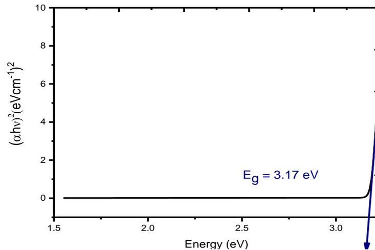
**Figure 3 (a)** The plot of extrapolation for TiO<sub>2</sub> nanoparticles from NaOH (0.1 g).
