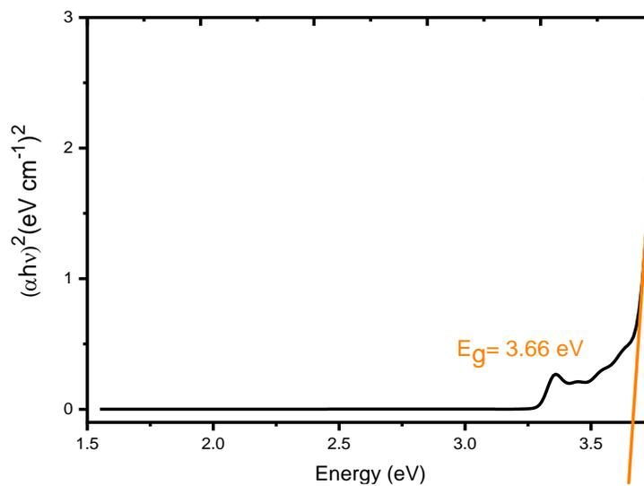
**Figure 3 (c)** The plot of extrapolation for TiO<sub>2</sub> nanoparticles from NaOH (0.5 g).
