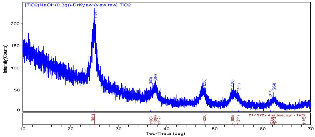
**Figure 1 (b)** XRD profiles of TiO<sub>2</sub> nanoparticles from NaOH(0.3g).
