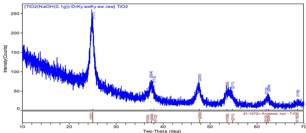
**Figure 1 (a)** XRD profiles of TiO<sub>2</sub> nanoparticles from NaOH(0.1g).
