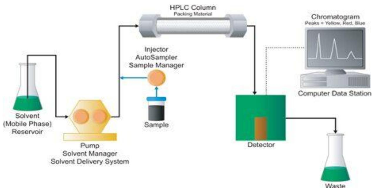
**Figure 4** Schematic Diagram of HPLC chromatogram at AIGLENT TECHNOLOGY
