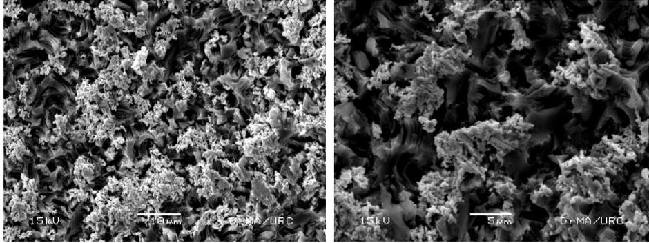
**Figure 13.** SEM photographs of porous formation using C7 method
