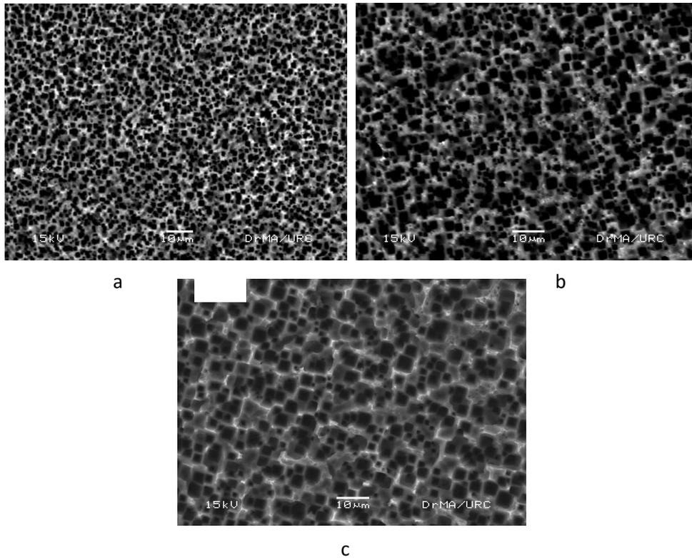
**Figure 16.** SEM photographs of porous size formation using C1 method for (a) 1 hour (b) 2 hours (c) 3 hours
