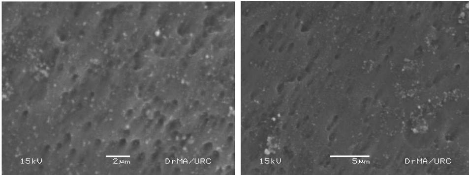
**Figure 12.** SEM photographs of porous formation using C6 method
