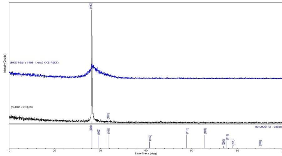
**Figure 18.** XRD characterizations of bulk silicon and porous silicon
