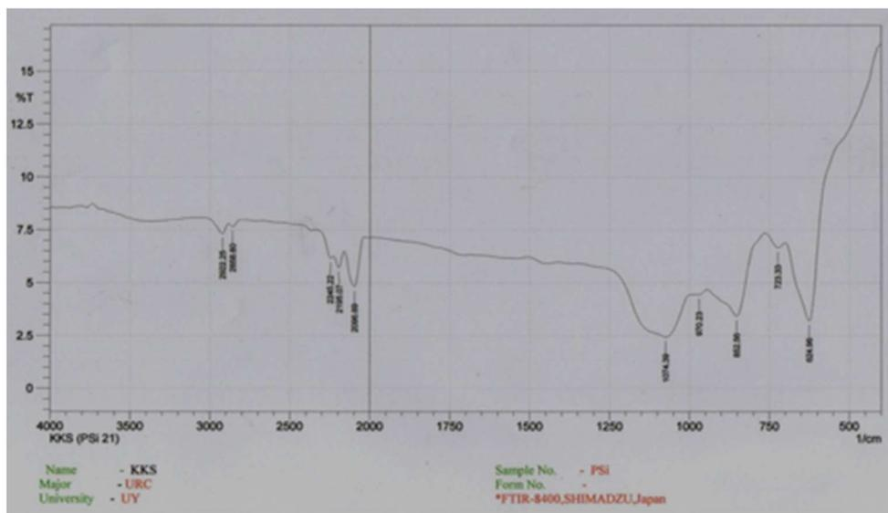
**Figure 19.** FTIR transmittance spectrum of a PS layer
