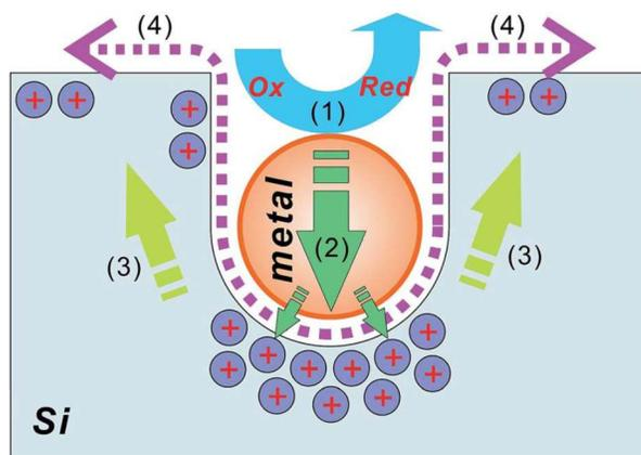
**Figure 1.** Illustration of the metal-assisted chemical etching process:
