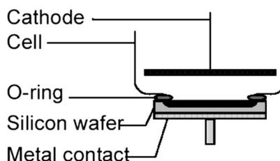
**Figure 3.** Schematic diagram for assembling of anodization
