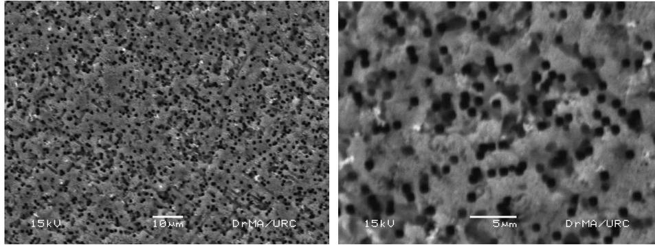
**Figure 10.** SEM photographs of porous formation using C4 method
