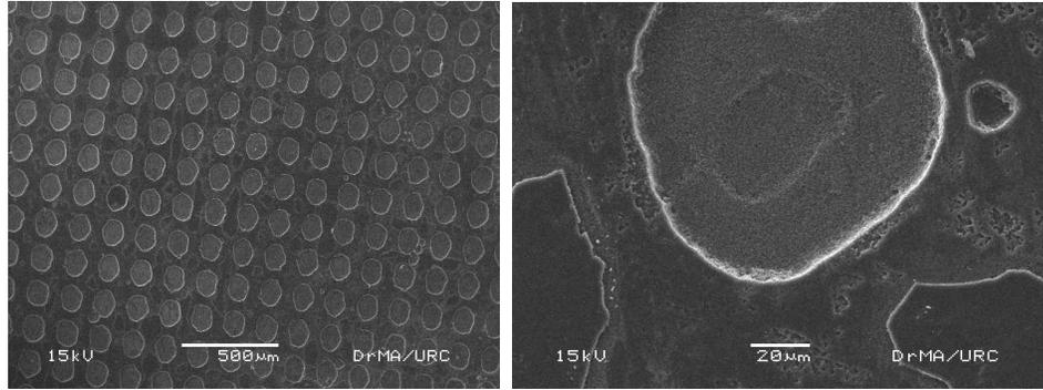
**Figure 17.** SEM photographs of porous formation using lithographic metal assisted chemical etching
