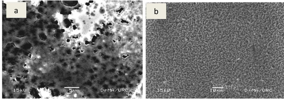
**Figure 4.** SEM photographs of porous formation using (a) A1 and (b) A2 method
