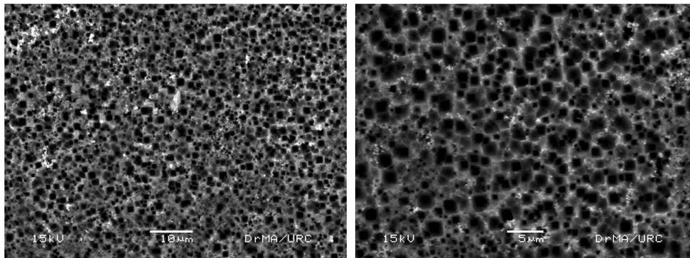
**Figure 8.** SEM photographs of porous formation using C2 method
