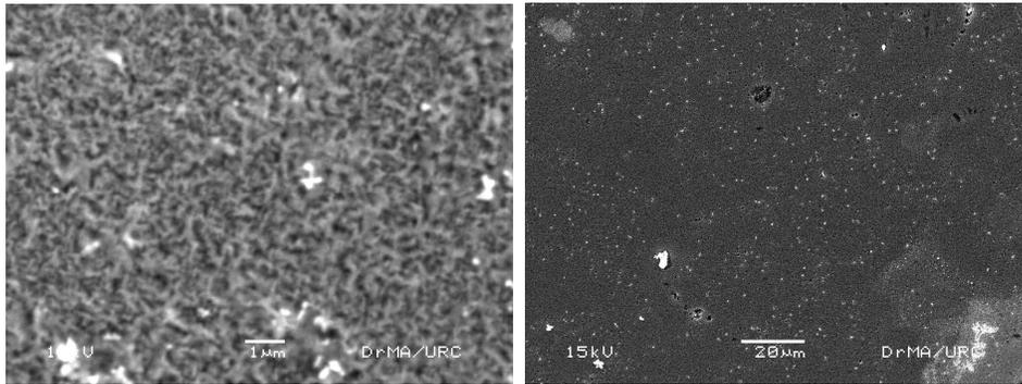
**Figure 14.** SEM images of porous formation using SDBE method
