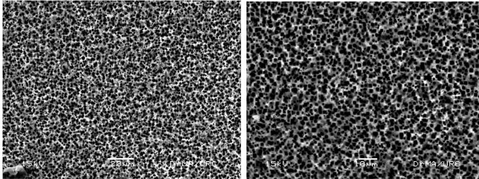
**Figure 7.** SEM photographs of porous formation using C1 method
