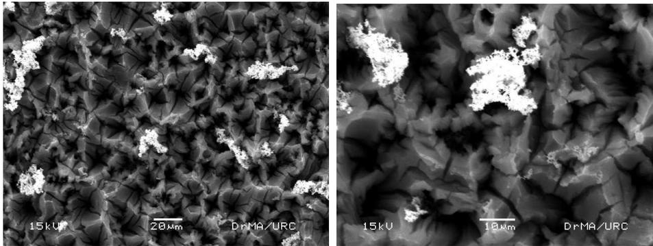
**Figure 11.** SEM photographs of porous formation using C5 method
