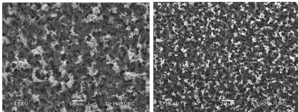
**Figure 9.** SEM photographs of porous formation using C3 method
