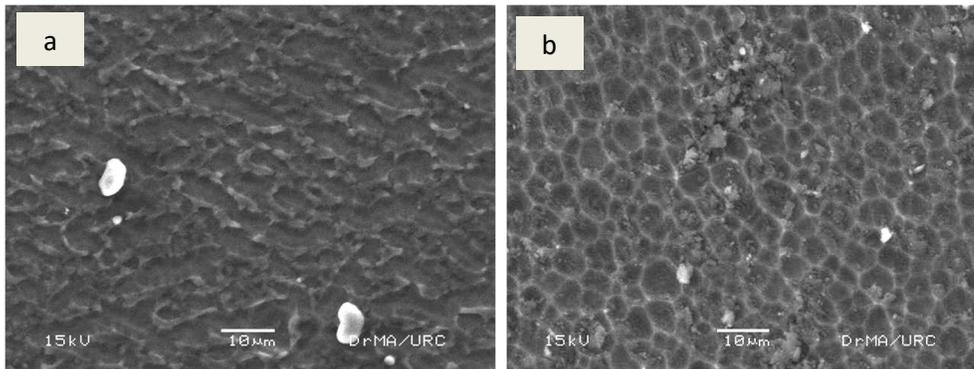
**Figure 5.** SEM photographs of porous formation using (a) A3 and (b) A4 method
