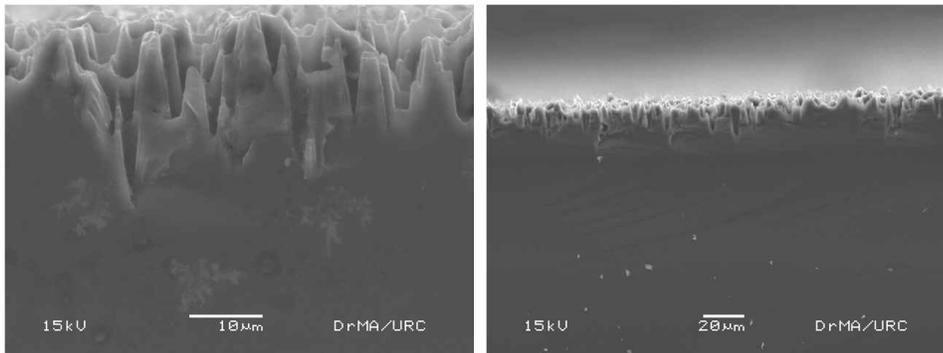
**Figure 15.** SEM images of porous thickness or pore length using C1 method after 3 hours etching time
