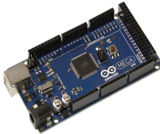
**Figure 2:** Photo of Arduino Mega 2560 microcontroller board
