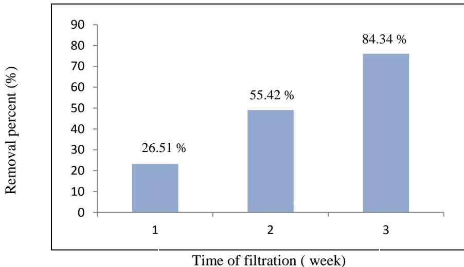
**Figure 6:** Plot of percent removal of lead vs time of filtration by using activated rice husk charcoal ( Site -1)
