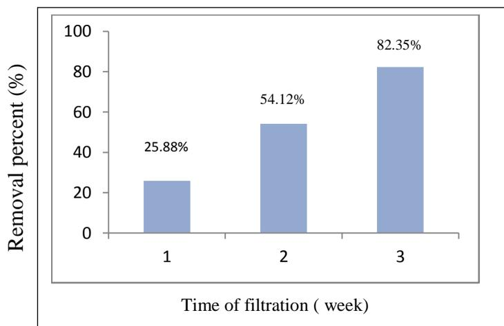
**Figure 7:** The plot of percent removal of lead vs time of filtration by using activated rice husk charcoal ( Site -2)
