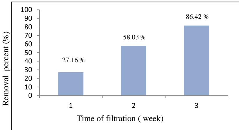
**Figure 8:** The plot of percent removal of lead vs time of filtration by using activated rice husk charcoal ( Site-3)
