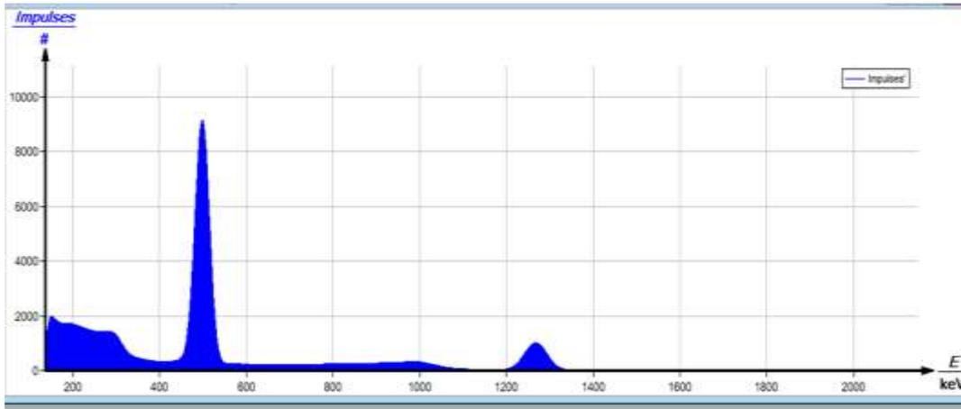
Figure 5 Typical  $^{22}\text{Na}$  spectrum measured using NaI(Tl) detector
