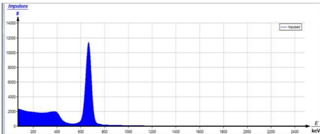
**Figure 3** Typical  $^{137}\text{Cs}$  spectrum measured using NaI(Tl) detector
