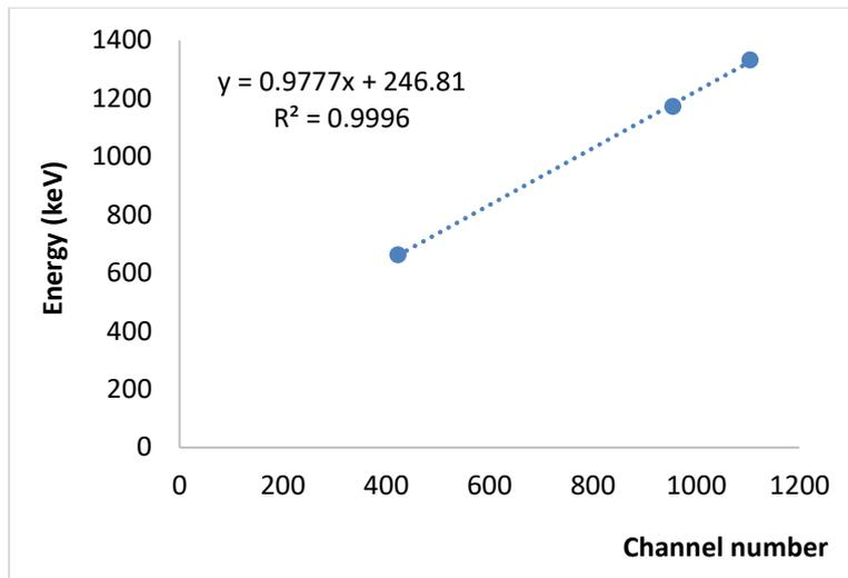
**Figure 2** The energy calibration curve for NaI(Tl) using  $^{60}\text{Co}$  and  $^{137}\text{Cs}$  nuclides
