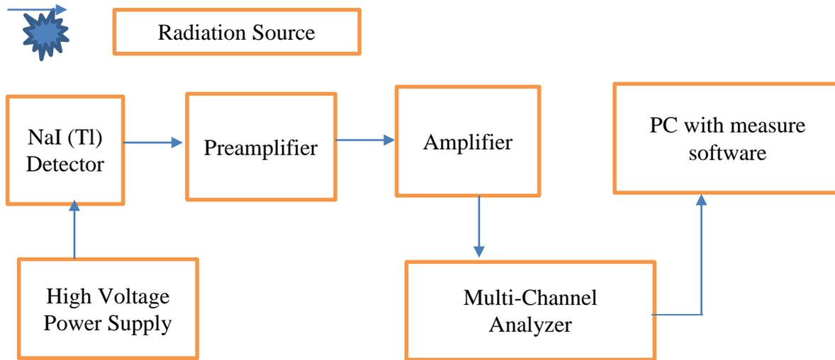
**Figure 1** Schematic diagram of the experimental setup
