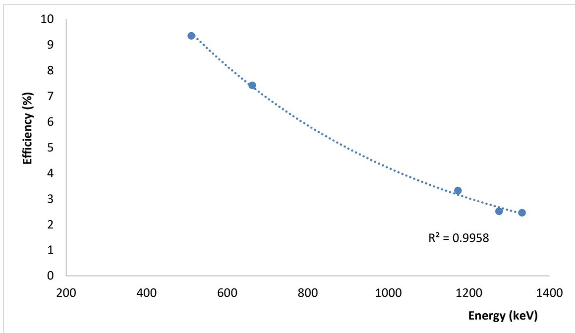
**Figure 6** Variation of detector efficiency as a function of different energies
