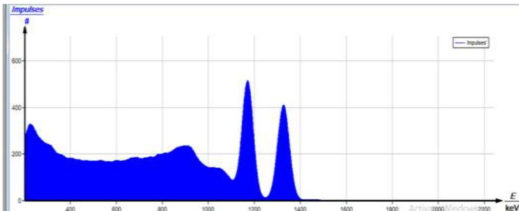
**Figure 4** Typical  $^{60}\text{Co}$  spectrum measured using NaI(Tl) detector
