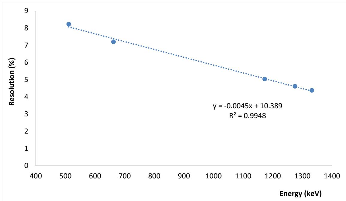
**Figure 7** Energy resolution of the NaI(Tl) detector
