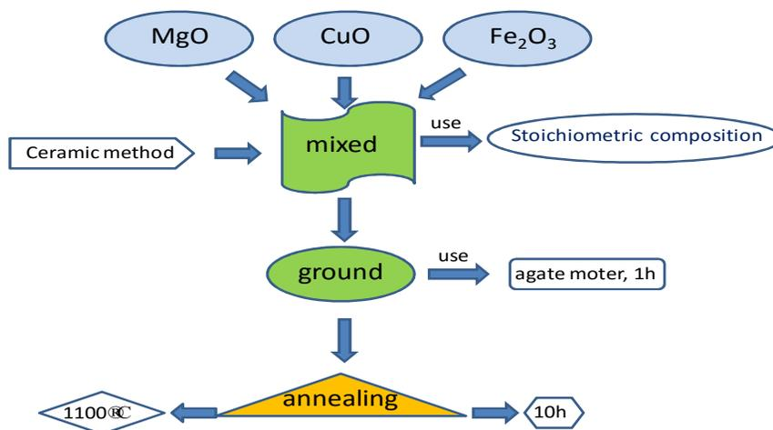
**Figure 1(c).** Flow diagram of the Mg-Cu ferrite sample preparation
