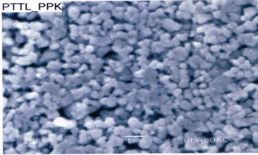
**Figure 6.** SEM image of Magnesium-Copper mixed ferrite,  $Mg_{0.5}Cu_{0.5}Fe_2O_4$
