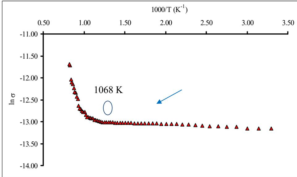
**Figure 7(a)** Arrhenius's plots of the conductivity with reciprocal temperature of the Magnesium-Copper mixed ferrite,  $Mg_{0.5}Cu_{0.5}Fe_2O_4$  (303 K – 1218 K)
