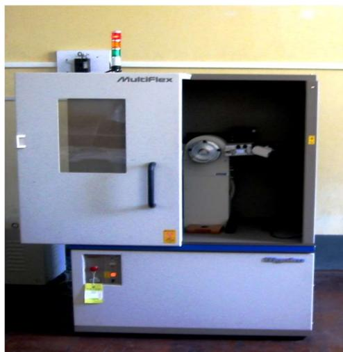
**Figure 2.** Photograph of the RIGAKU MULTIFLEX X-Ray Diffractometer
