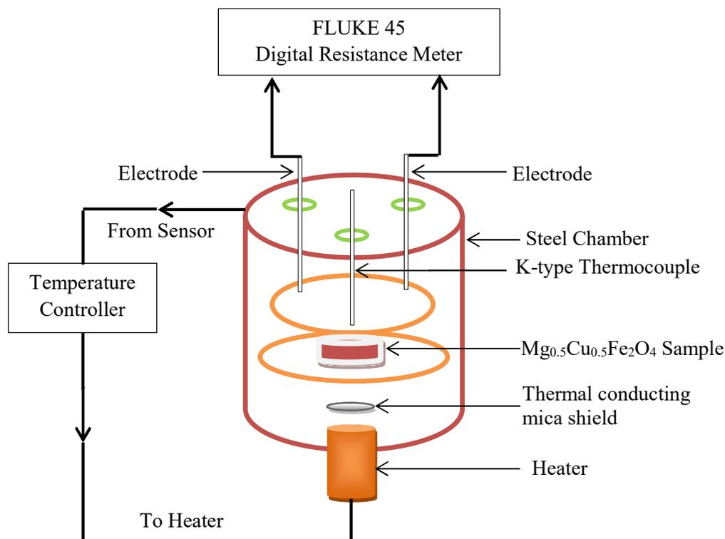
**Figure 4(b).** Sample chamber for temperature dependent electrical resistance measurement
