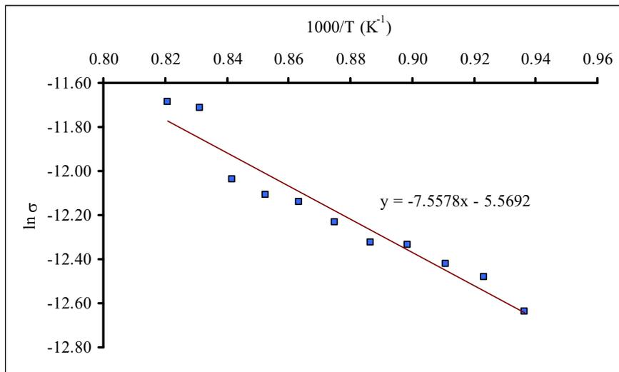
**Figure 7(b)** Arrhenius's plots of the conductivity with reciprocal temperature of the Magnesium-Copper mixed ferrite,  $Mg_{0.5}Cu_{0.5}Fe_2O_4$  (1068 K – 1218 K)
