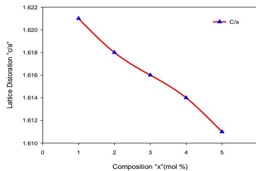
**Figure 4** Influence of composition " x " (mol %) on lattice distortion " c/a " of ZnO structure.
