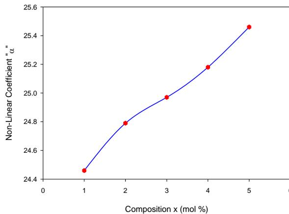
**Figure 8** Influence of composition " x " (mol %) on the non - linearity factor "  $\alpha$  " of prepared varistors.
