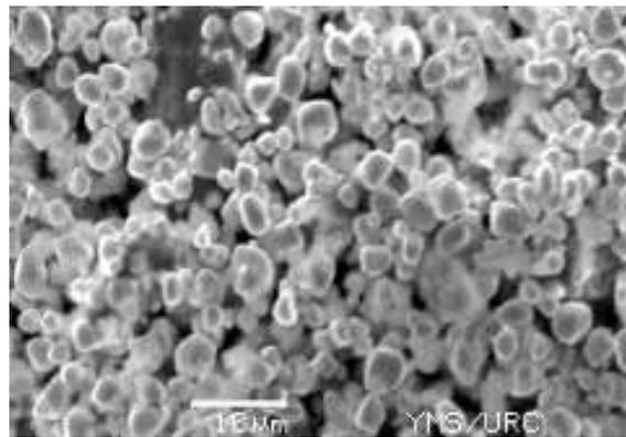
**Figure 6(e)** The SEM Images of ZnO based Varistor with five additive oxide (composition  $x = 0.05$ )
