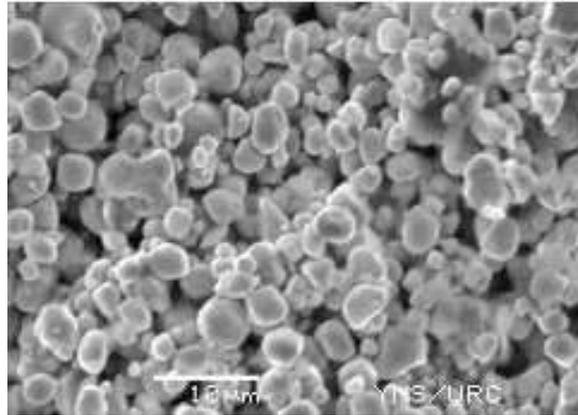
**Figure 6(d)** The SEM Images of ZnO based Varistor with five additive oxide (composition  $x = 0.04$ )
