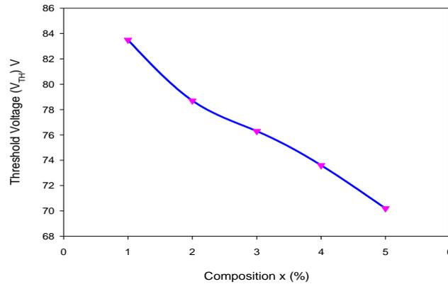
**Figure 9** Variation of composition " x " (mol %) with threshold voltage ( $V_{TH}$ ) of prepared varistors.
