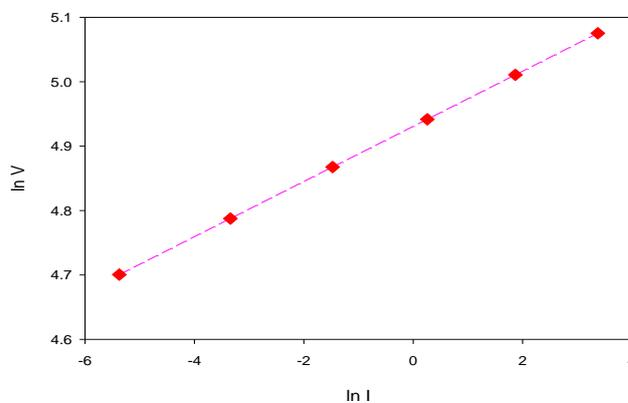
**Figure 7(a)** Non- linear behavior of ZnO based Varistor with five additive oxide (composition  $x = 0.01$ ).
