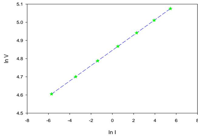
**Figure 7(b)** Non- linear behavior of ZnO based Varistor with five additive oxide (composition  $x = 0.02$ ).
