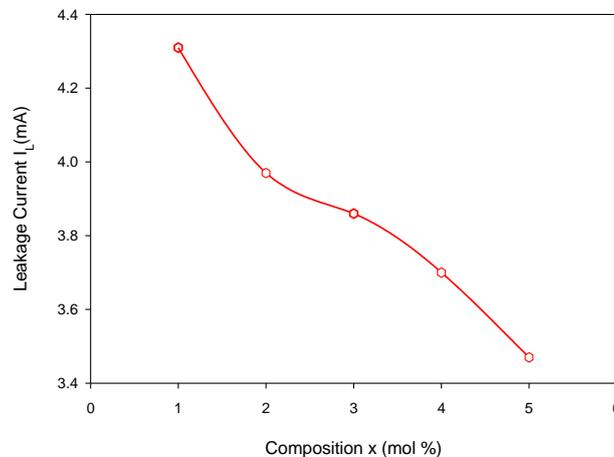
**Figure 10** Effect of composition " x "(mol %) on leakage current "  $I_L$  " of prepared varistors.
