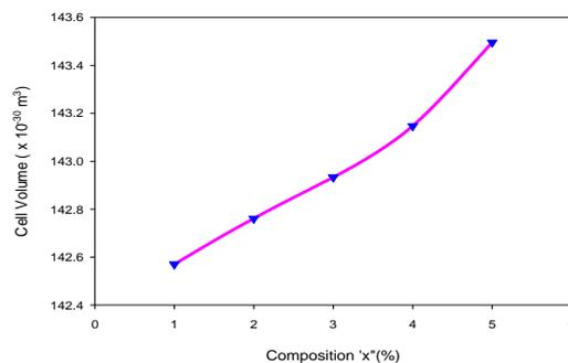
**Figure 5** Effect of composition " x " (mol %) on unit cell volume of ZnO structure.
