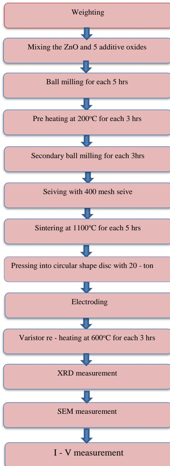
**Figure 1** Flow diagram of experimental.
