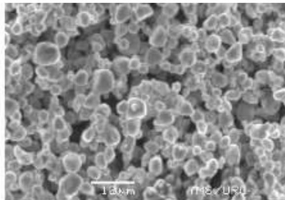
**Figure 6(c)** The SEM Images of ZnO based Varistor with five additive oxide (composition  $x = 0.03$ )
