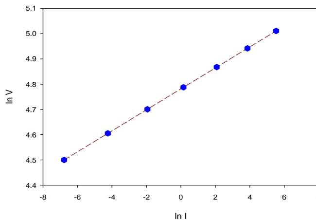
**Figure 7(d)** Non- linear behavior of ZnO based Varistor with five additive oxide (composition  $x = 0.04$ )
