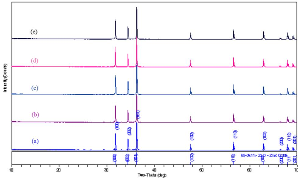
**Figure 2** XRD spectra of ZnO with five additive oxides (composition 'x'= 1 mol%, 2 mol%, 3 mol%, 4 mol% and 5 mol%).
