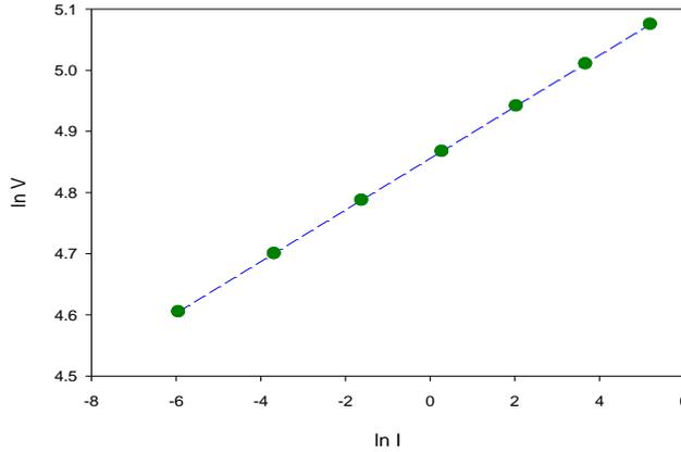
**Figure 7(e)** Non- linear behavior of ZnO based Varistor with five additive oxide (composition x = 0.05).
