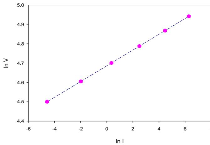
**Figure 7(c)** Non- linear behavior of ZnO based Varistor with five additive oxide (composition  $x = 0.03$ ).
