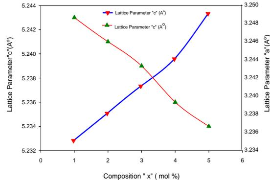
**Figure 3** Variation of composition " x " (mol %) with the lattice constants of ZnO structure.
