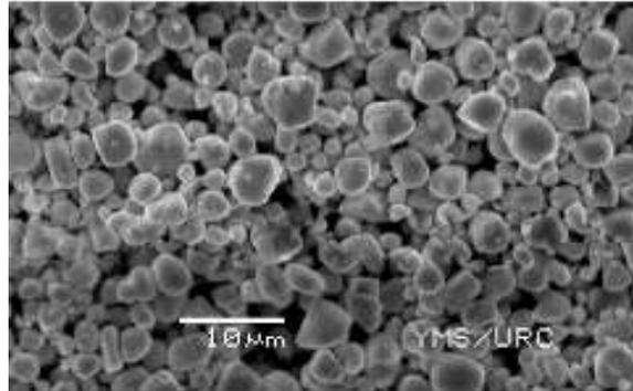
**Figure 6(a)** The SEM Images of ZnO based Varistor with five additive oxide (composition  $x = 0.01$ )
