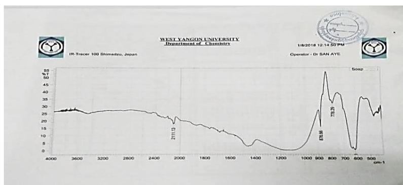
Figure 5 FT IR spectrum of natron (purified)
