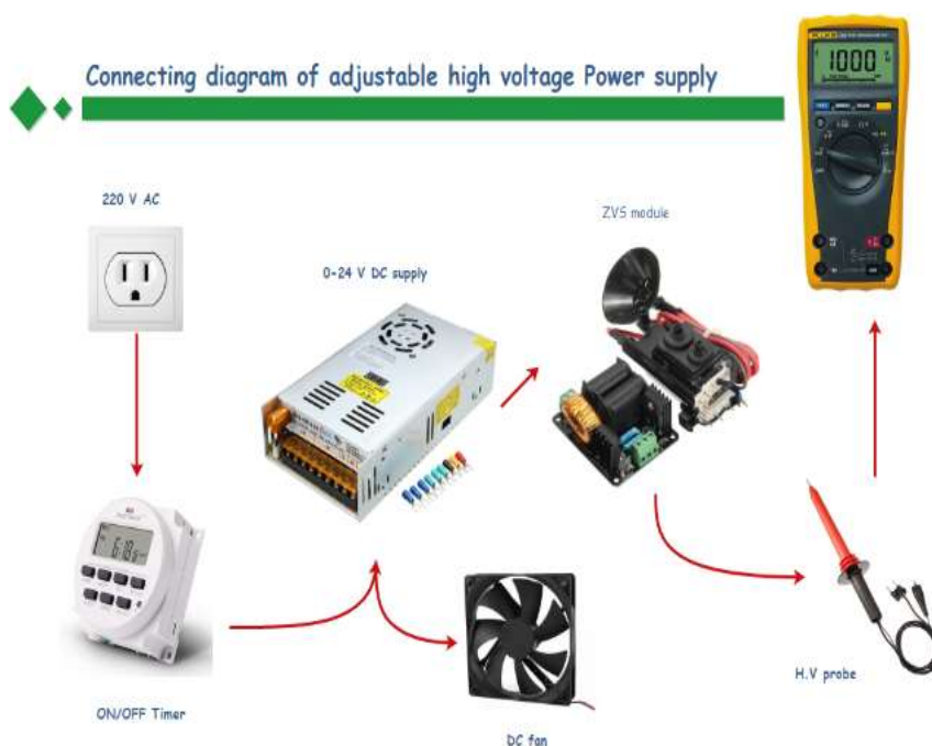
Figure 1 (a) The connecting diagram of automatic on/off variable HV power supply
