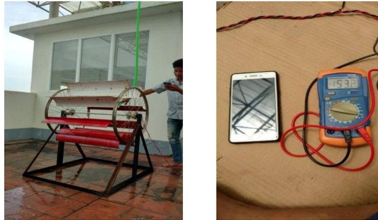
**Figure 9** Test run of flow turbine by 1-inch pipe and 10 feet height
