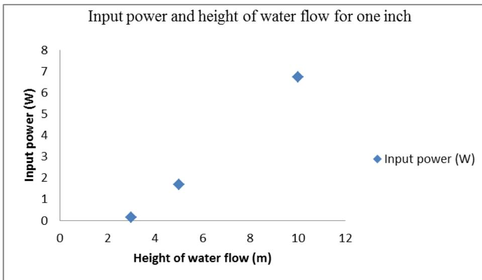
**Figure 10** Input power depend on height of water flow with one-inch pipe
