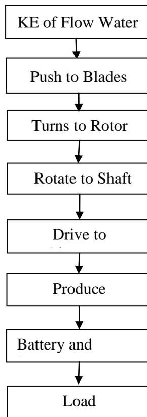
**Figure 1** The working procedure of flow turbine
