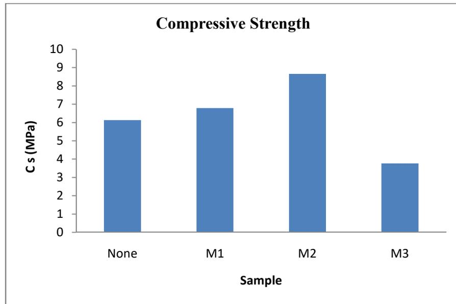
**Figure 9** Compressive strength vs different fibres content
