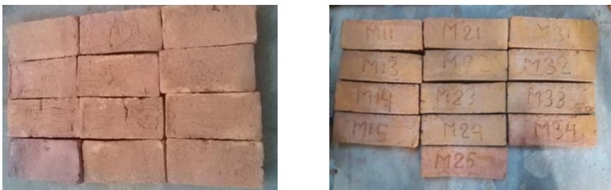
**Figure 3**Bricks for measuring the compressive and bending strength
