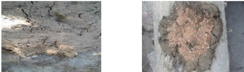
**Figure 1**Sawdust (Wood-fibres) with clay mixture
