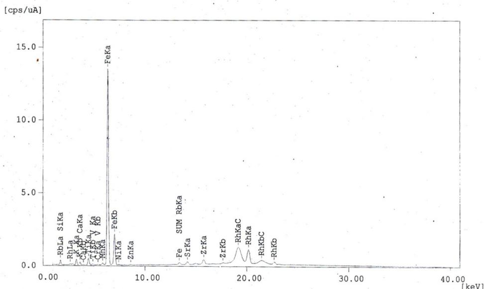
**Figure 6** EDXRF pattern for sample S2
