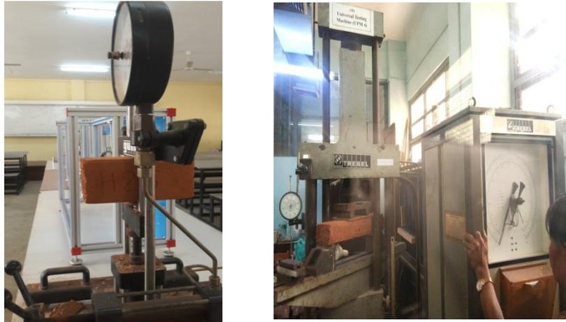
Figure 4 Compressive and bending strength testing machines
