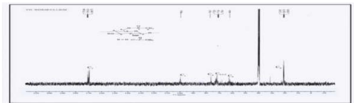
**Figure 9**  $^{13}\text{C}$  NMR spectrum of wheat straw cellulose acetate (WSCA-1)
