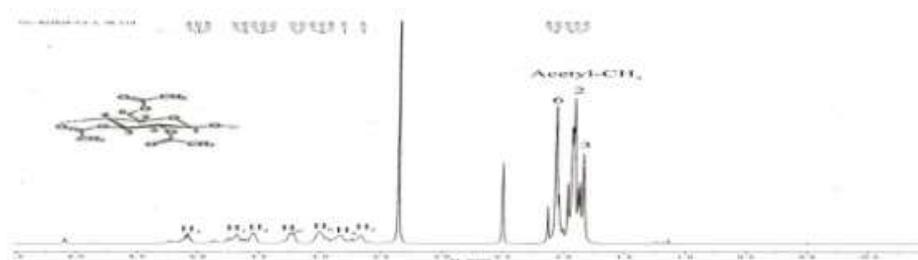
**Figure 7.  $^1H$  NMR spectrum of wheat straw cellulose acetate (WSCA-1)**
