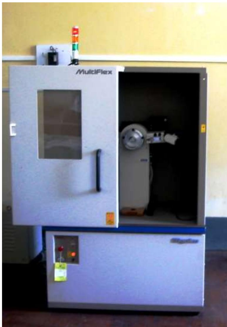
**Figure 1** Diagram of XRD Rigaku Multiflex.
