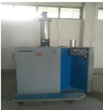
**Figure 2:** Photograph of Co-60 gamma chamber 5000
