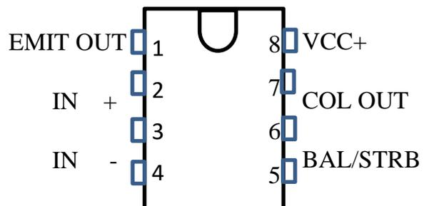
**Figure 4** Component of LM311 comparator and pin out diagram
