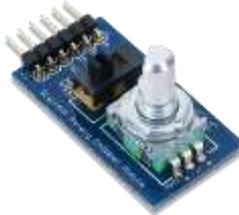
**Figure 2** Component of rotary encoder module
