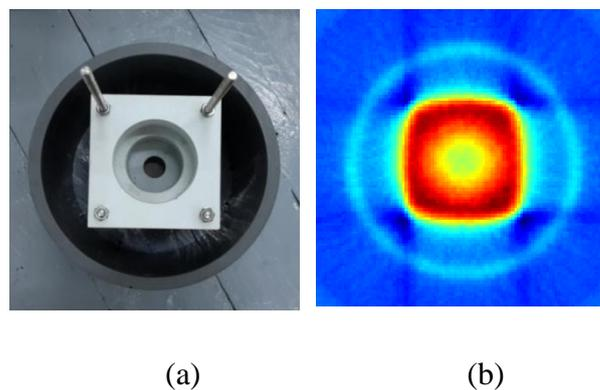
**Figure 10**The comparison of (a) the optical camera image and (b) the reconstructed cross-sectional image of the internal structure of the lead block
