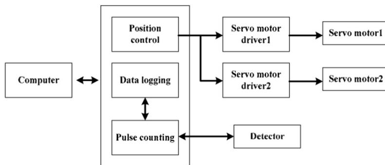
**Figure 6** The block diagram of the operation of the CT system
