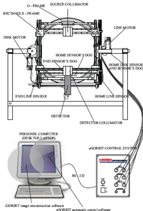
**Figure 3** General arrangement of whole GORBIT system
