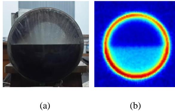
**Figure 11** The comparison of (a) the optical camera image and (b) the reconstructed cross-sectional image of the phase distribution in the pipe
