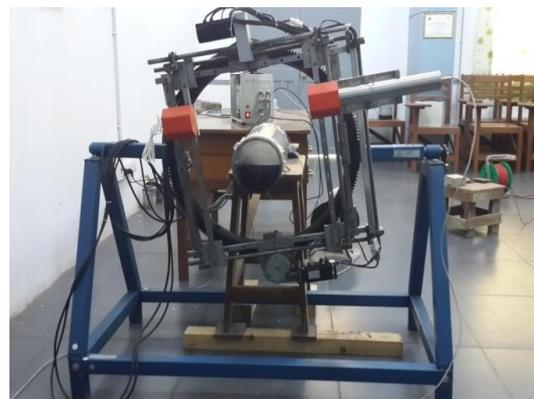
**Figure 5** The vertical arrangement for the measurement of the phase distribution in the pipe
