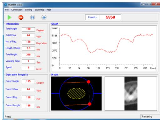
**Figure 7** The parameters for automatic scan by using eGORBIT software
