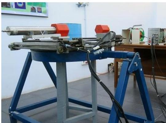
**Figure 4** The horizontal arrangement for the measurements of different density and internal structure of the objects
