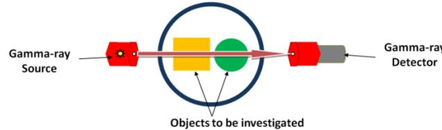
**Figure 1** Schematic principle of gamma computed tomography(CT) system
