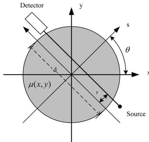
**Figure 2** Arrangement of a transmission CT scanning system
