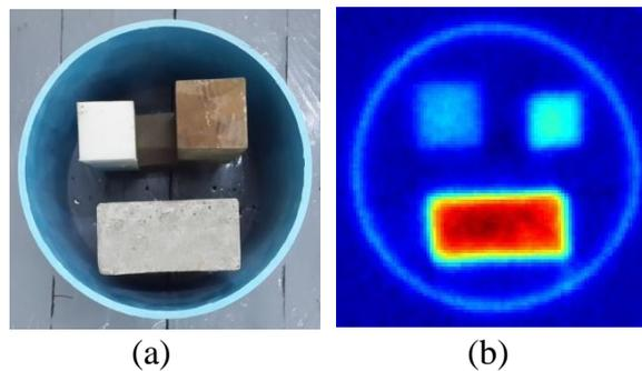
**Figure 9** The comparison of(a) the optical camera image and (b) the reconstructed cross-sectional image of the interior density distribution of different density objects
