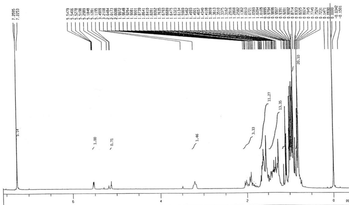
Figure 4 <sup>1</sup>H NMR (400 MHz in CDCl<sub>3</sub>) spectrum of isolated compound (Lupeol)
