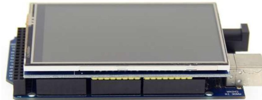
**Figure 5** The LCD is connected with Arduino Mega2560 board
