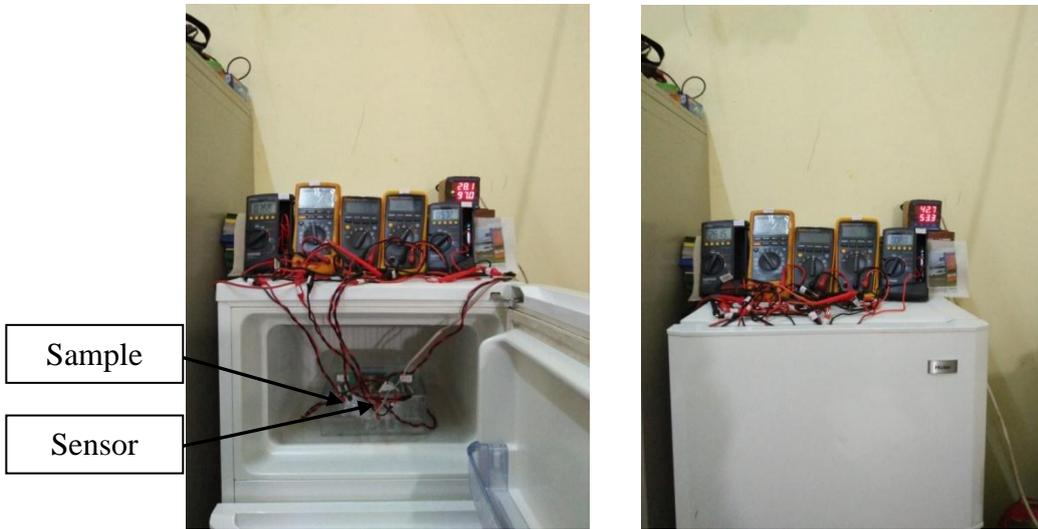
**Figure 3** Experimental setup of humidity sensitive electrical resistance measurements, (a) the sample and sensor placed in the same condition (altitude) and (b) wiring connection of sample and resistance meter
