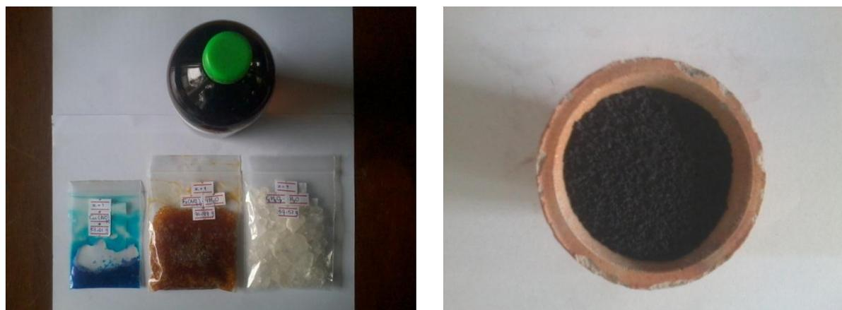
**Figure 1** Photographs of (a) the weighed starting materials and (b) as-burnt  $\text{Cu}_x\text{Co}_{1-x}\text{Fe}_2\text{O}_4$  for  $x = 1.00$
