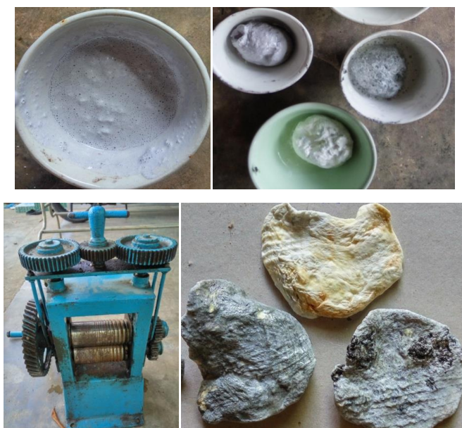
Figure 3 : The photograph of preparation of rubber ferrite matrices.
