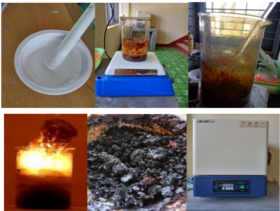
Figure 2 : The photograph of preparation of ferrites powder.
