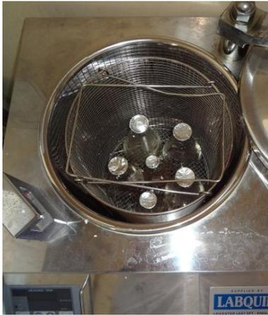
(c) Placing in the autoclave
