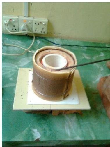
(e) Home-made furnace and temperature sensor
