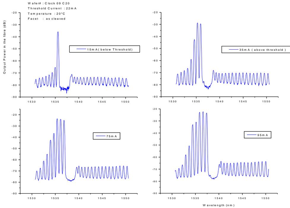
**Figure-2** Lasing spectra of Index-Coupled DFB laser with cleaved facets.
