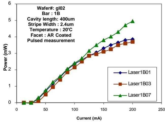
**Figure 8** Light output versus current characteristics of Gain-Coupled DFB laser with AR-coated facets.
