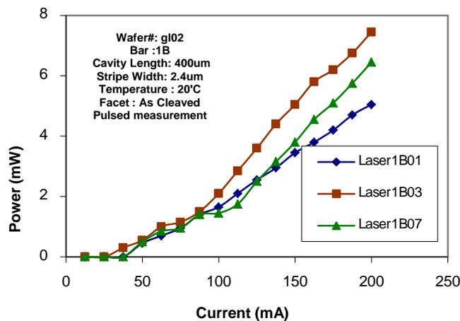
**Figure 6** Light output versus current characteristic of Gain-Coupled DFB laser with cleaved facets.
