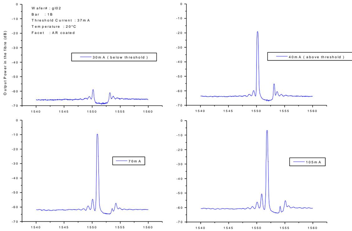
**Figure 9** Lasing spectra of Gain-Coupled DFB laser with AR-coated facets.
