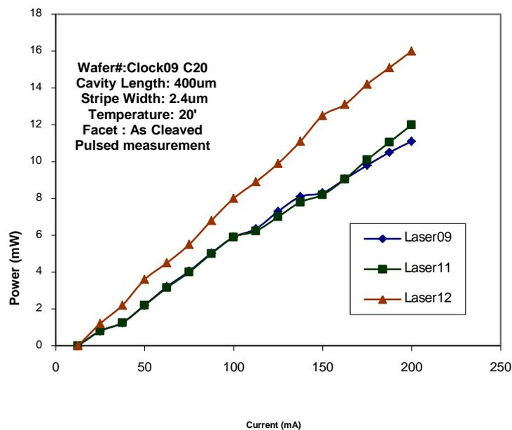
**Figure 1** Light output versus current characteristics of Index-Coupled DFB laser with cleaved facets.
