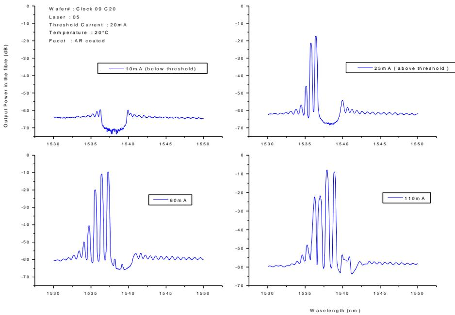
Figure 4 Lasing spectra of Index-Coupled DFB laser with AR-coated facets.
