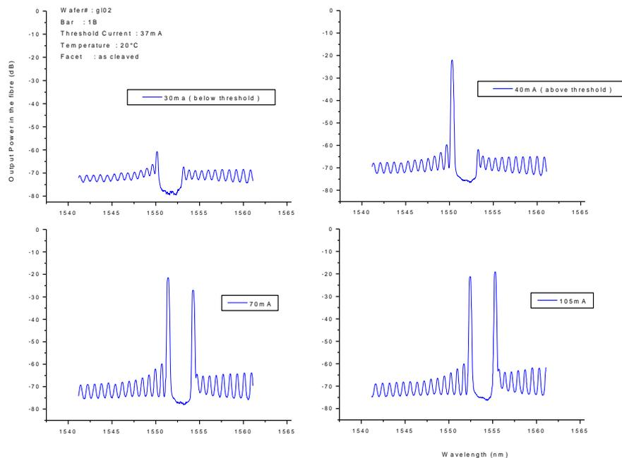
**Figure 7** Lasing spectra of Gain-Coupled DFB laser with cleaved facets.
