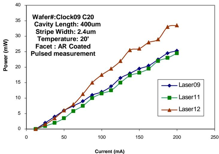
**Figure 3** Light output versus current characteristic of Index-Coupled DFB laser with AR-coated facets.
