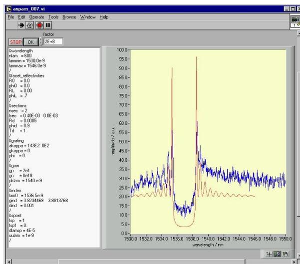
Figure 5 Theoretical curve fitting with the experimental result of the Index-Coupled DFB laser.
