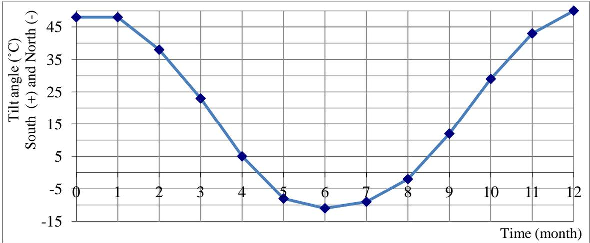
**Figure 1.12** Determination of monthly optimum tilt angle for Minbu solar power plant
