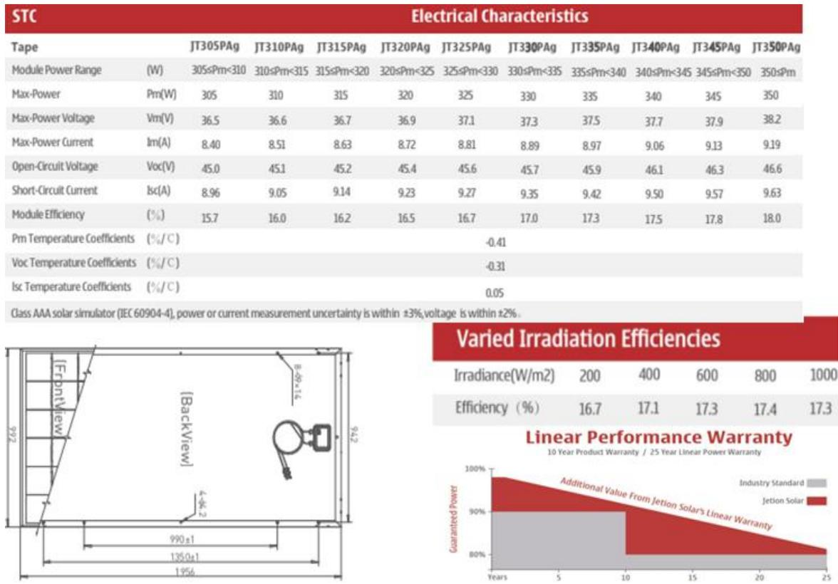
Figure 1.6 Specification of solar panel (JT310) of Minbu solar power plant.
