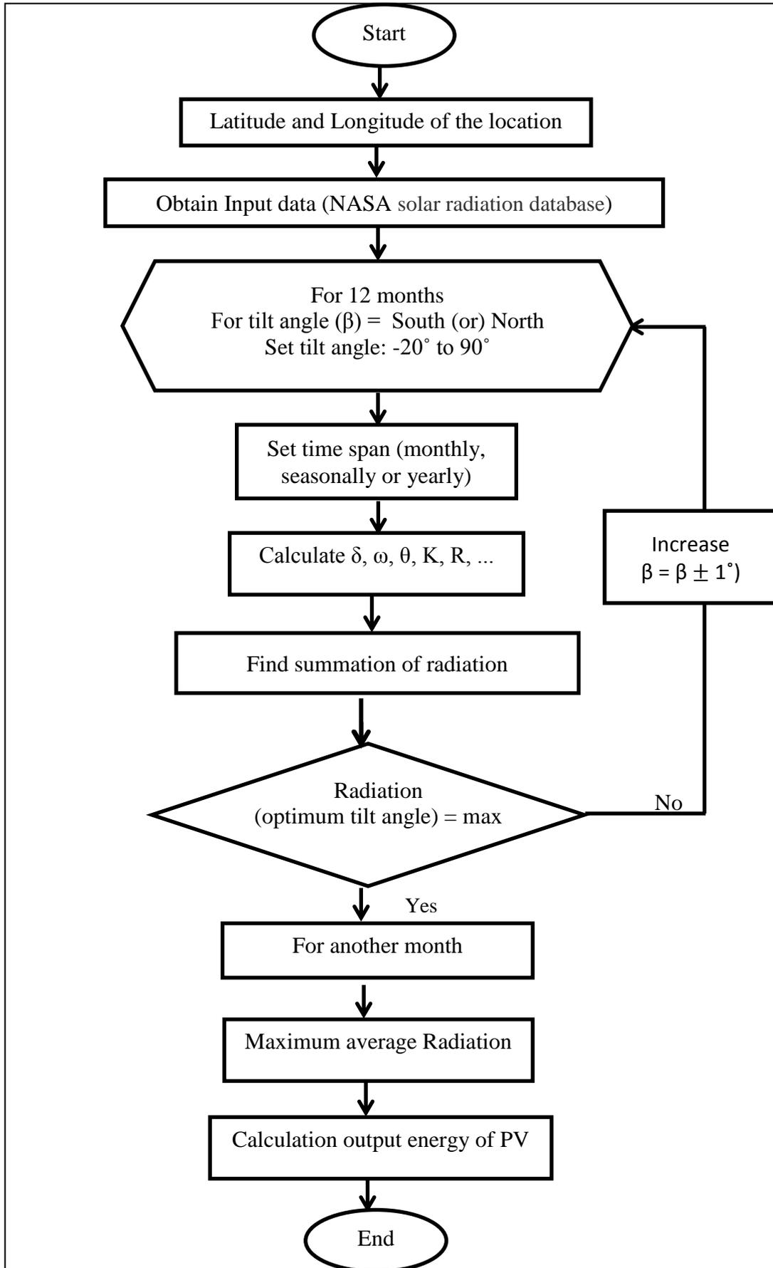
Figure 1.7 Optimization algorithm for PV panels tilt angle.
