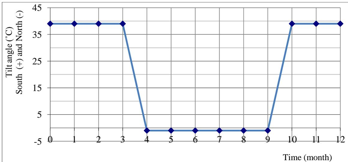
Figure 1.11 Determination of seasonally optimum tilt angle for Minbu solar power plant.
