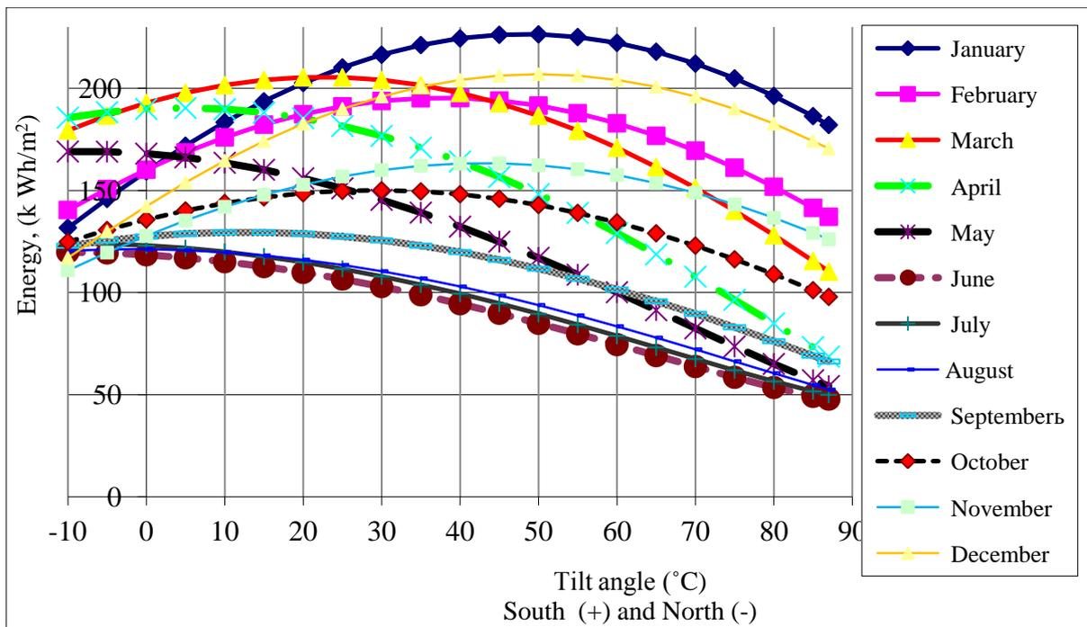
**Figure 1.13** Monthly tilt angle optimization results (solar radiation and tilt angle) for Minbu solar power plant
