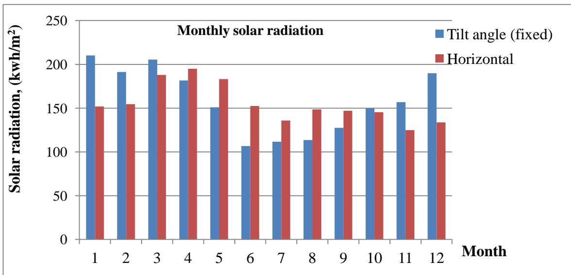
Figure 1.10 (a) Solar radiation for optimum tilt angle for Minbu solar power plant.
