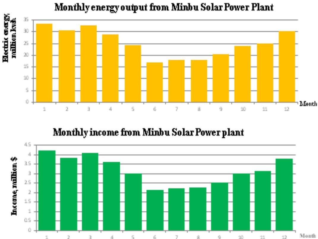
Figure 1.15 Energy output and income of Minbu Solar Power Plant (170 MW).
