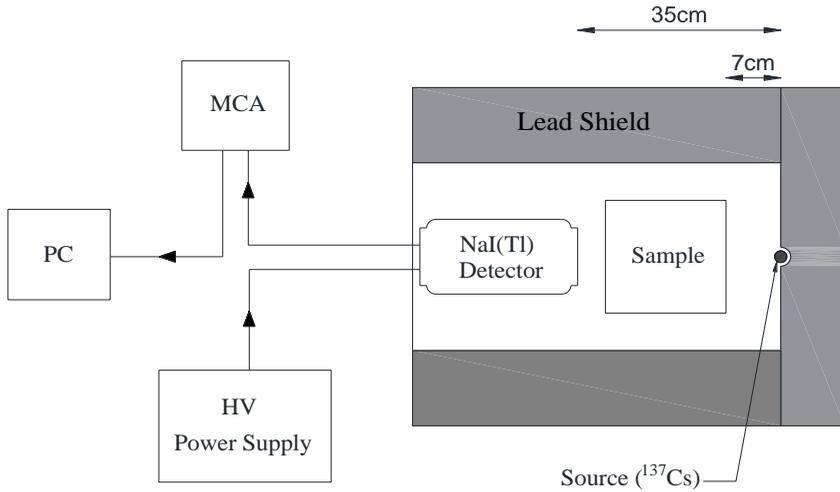
**Figure 1:** Block diagram of Experimental Set up
