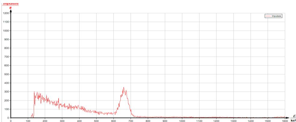
**Figure 4:** The recorded spectrum of AAC block sample for  $^{137}\text{Cs}$  source with absorber thickness 24.1cm
