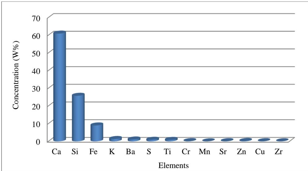
**Figure 2:** Elemental Concentrations in AAC Block Sample
