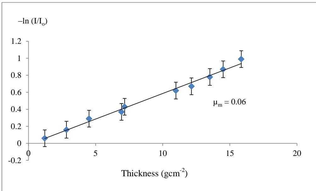
**Figure 6:**  $-\ln(I/I_0)$  versus different thicknesses (gcm<sup>-2</sup>) of AAC block sample of  $^{137}\text{Cs}$  source
