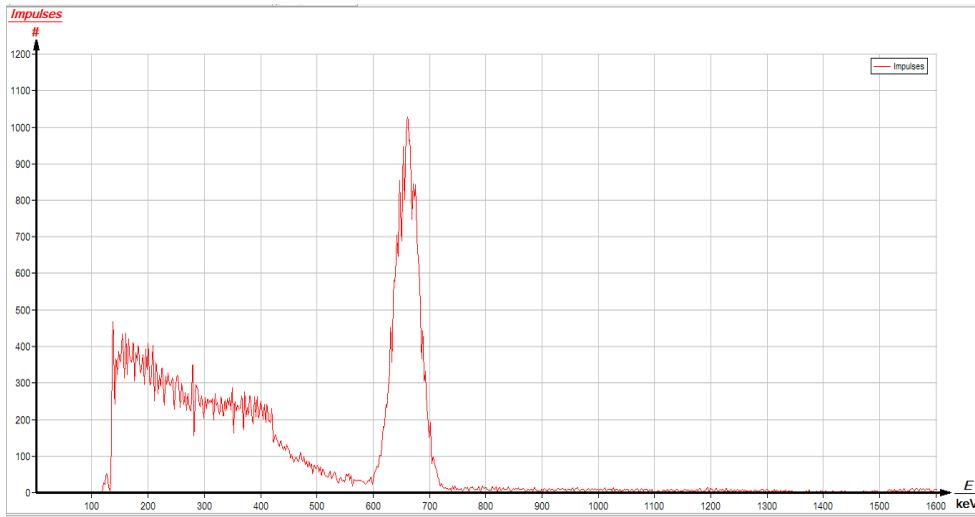
**Figure 3:** The recorded spectrum of AAC block sample for  $^{137}\text{Cs}$  source without absorber
