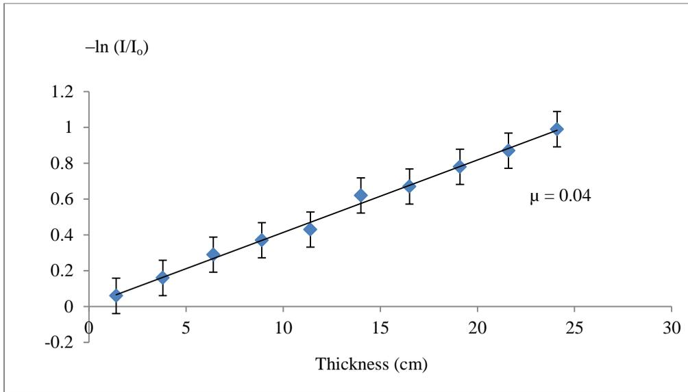
**Figure 5:**  $-\ln(I/I_0)$  versus different thicknesses (cm) of AAC block sample of  $^{137}\text{Cs}$  source
