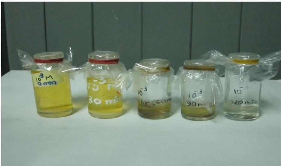
**Figure 12:** Photo of degradation of methyl orange by Ag/TiO<sub>2</sub> film after dipping for 3s in 0.001 M of silver solution during 2 hours.
