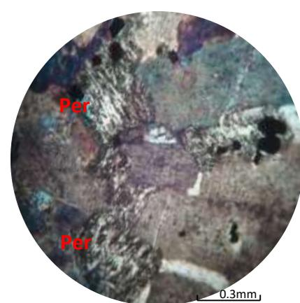
**Figure 6** String perthite in hornblende biotite granodiorite, between XN
