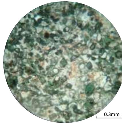
**Figure 14** Ocellar texture of dolerite, between XN
