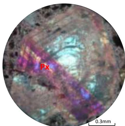
**Figure 5** Sector-zoned and each sector displays oscillatory zoning of pyroxene in gabbro, between XN
