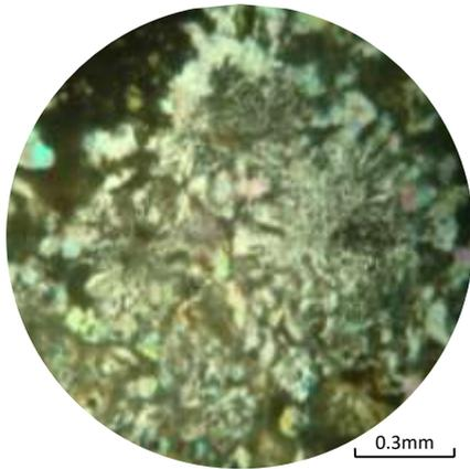
**Figure 13** Myrmekitic texture in leucogranodiorite, between XN
