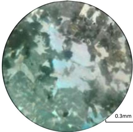
**Figure 7** Consertal texture in hornblende - biotite granodiorite, between XN
