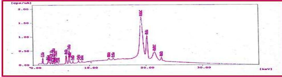
**Figure 12:** The X-ray fluorescence analysis for Rice Husk Ash in Hlaegu for 2 hours at 700°C
