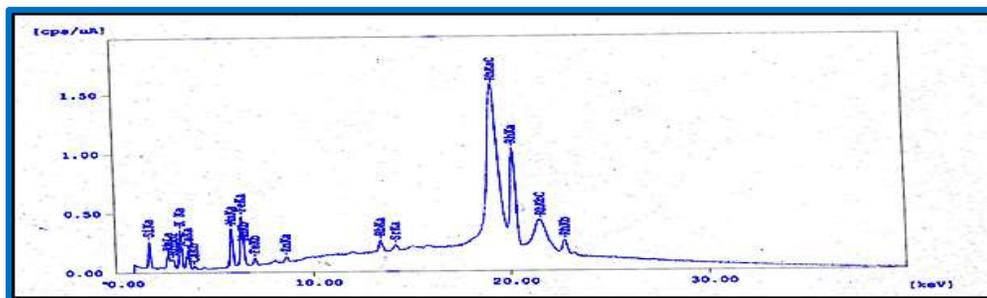
**Figure 11:** The X-ray fluorescence analysis for Rice Husk Ash in Hlaegu for 2 hours at 600°C
