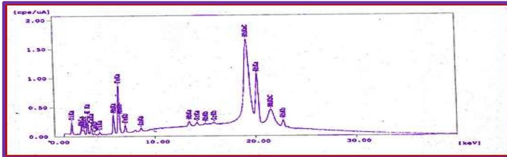
**Figure 13:** The X-ray fluorescence analysis for Rice Husk Ash in Hlaegu for 2 hours at 800°C
