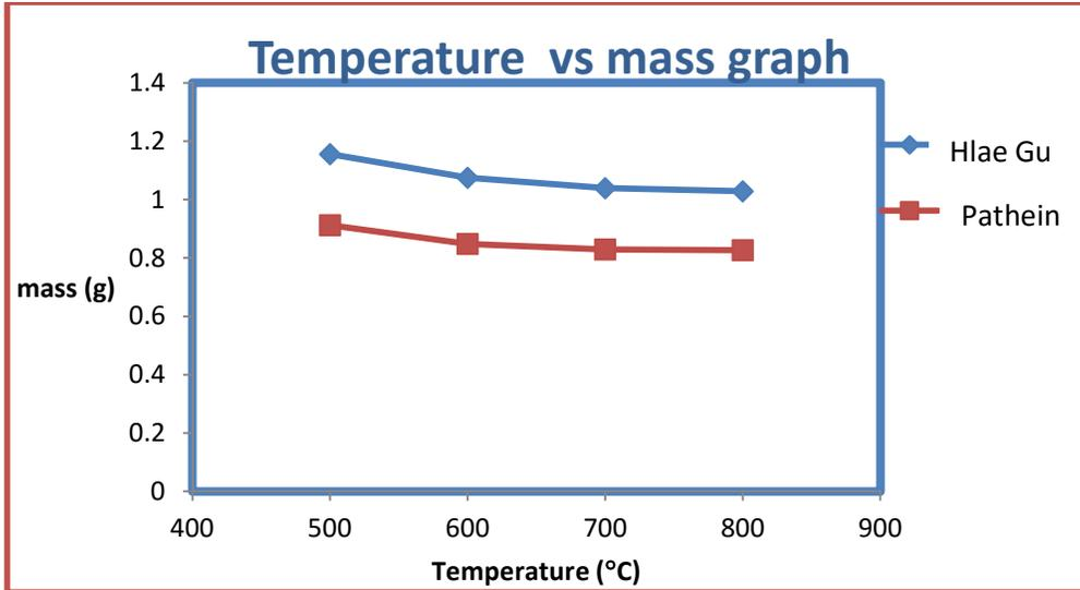
**Figure 8:** The different mass of RHA from rice husk calcined at different temperature
