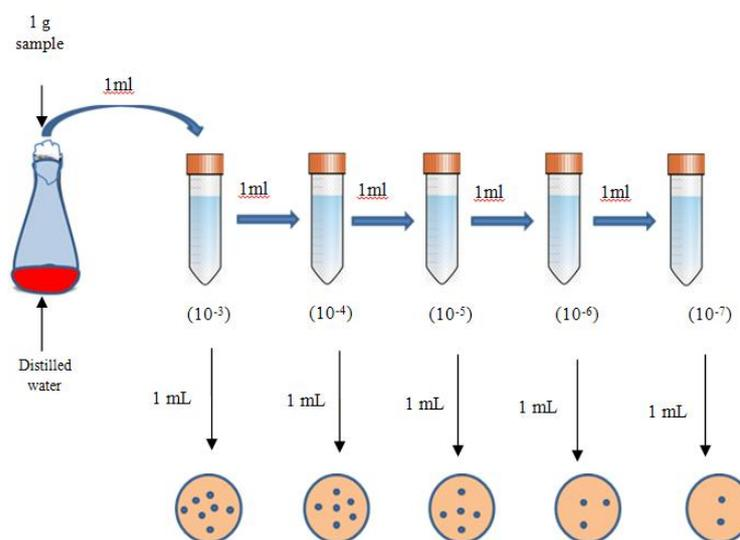
**Figure 1** Serial dilution method for soil samples (Collin, 1964)
