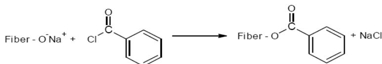
When benzoyl chloride reacts with areca fibers, an ester linkage is formed. This benzoyl chloride treatment results in the reduction of hydrophilicity of areca fibers and hence made the areca fibers to become more compatible with polymer matrix. Benzoylation treatment also enhances thermal stability of the fibers. These could improve chemical interlocking at the interface and provides effective fiber surface area for good adhesion with the matrix (Dhanalakshmi *et al.*, 2015).
