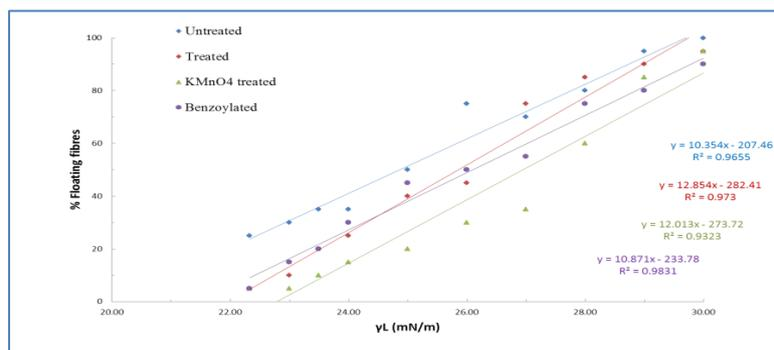
**Figure 6** Plot of percent of floating fibres as a function of surface tension of water-methanol mixtures
