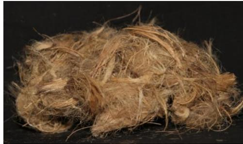
Figure 2 Extracted areca nut fibre
