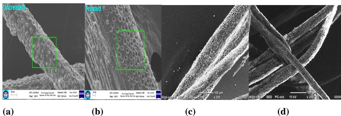
**Figure 3** SEM micrographs of the areca nut fibre (a) untreated (b) alkali treated (c) permanganate treated and (d) benzoyl chloride treated
