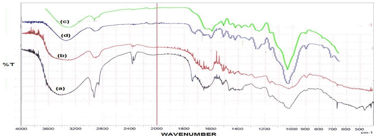
**Figure 4** FT IR spectra of areca nut fibre (a) untreated (b) alkali treated (c) permanganate treated and (d) benzoyl chloride treated
