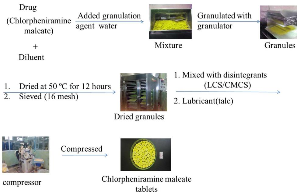
**Figure 2.** Determination of the Starch and its Derivative in Procedure for Tablet Manufacturing Process
