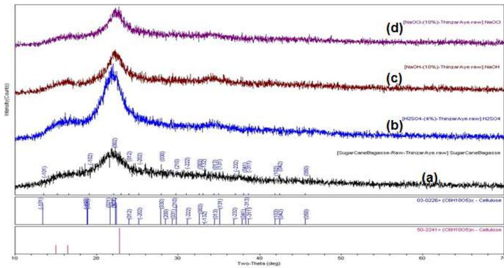
**Figure 6:** XRD patterns of (a) sugar cane bagasse raw sample (b) acid treated sample (c) base treated sample and (d) cellulose fiber
