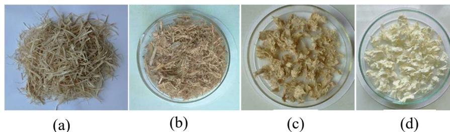
**Figure 2:** (a) Sugar cane bagasse raw sample (b) acid treated sample (c) base treated sample and (d) cellulose fiber
