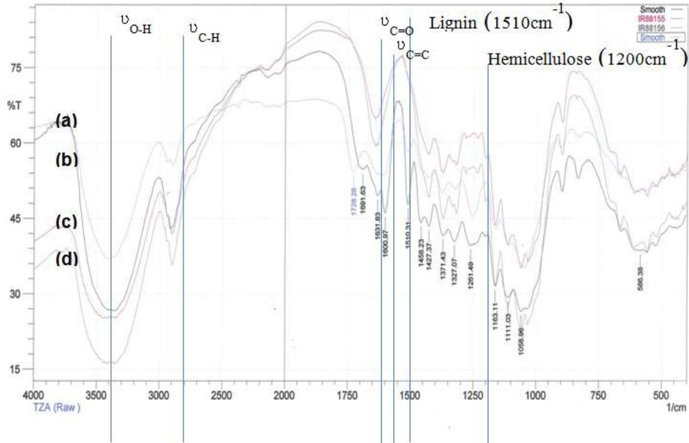
**Figure 4:** FTIR spectra of (a) sugar cane bagasse raw sample (b) acid treated sample (c) base treated sample and (d) cellulose fiber
