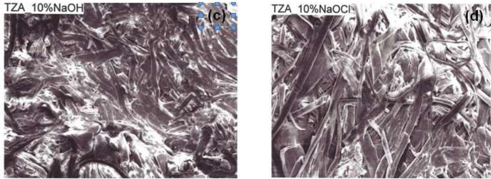
**Figure 5:** SEM photographs of (a) sugar cane bagasse raw sample (b) acid treated sample (c) base treated sample and (d) cellulose fiber
