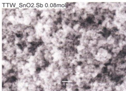
**Figure 2:**(d) SEM photo graph of Sb (8 mol% SnO<sub>2</sub>)
