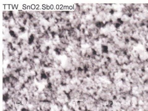
**Figure 2:** (a). SEM photo graph of Sb (2 mol% SnO<sub>2</sub>)
