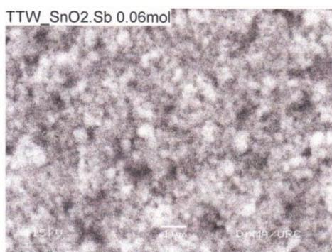
**Figure 2:** (c). SEM photo graph of Sb (6 mol% SnO<sub>2</sub>)
