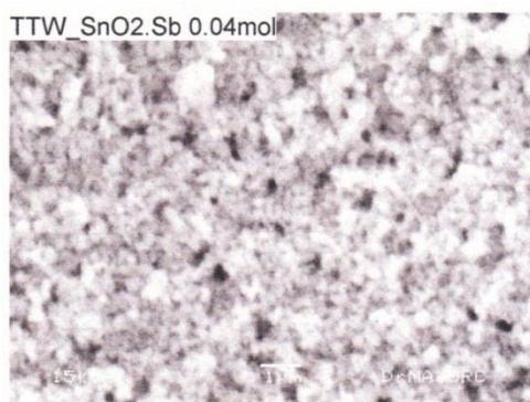
**Figure 2:** (b). SEM photo graph of Sb (4 mol% SnO<sub>2</sub>)
