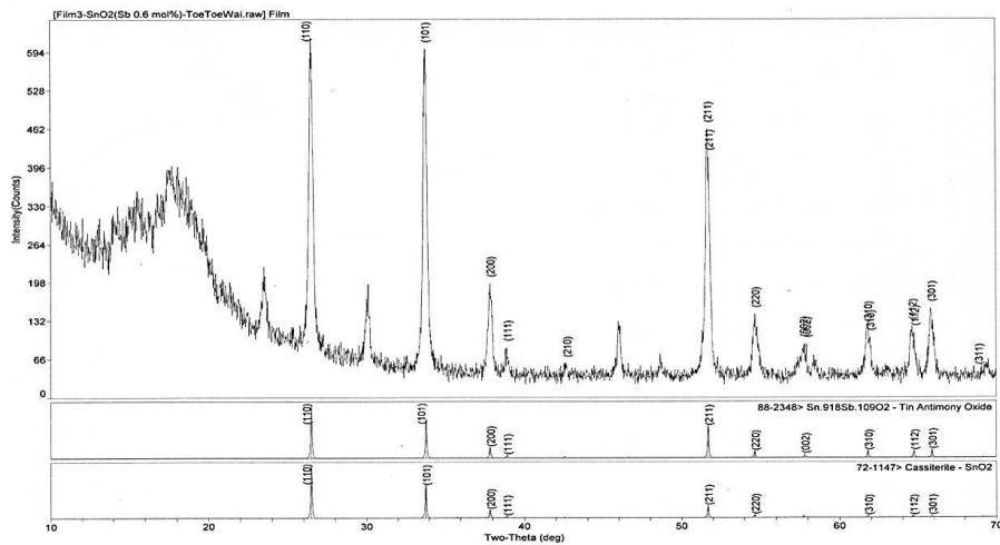
**Figure 1:** (c) XRD patterns obtained for Sb(6 mol% SnO<sub>2</sub>)
