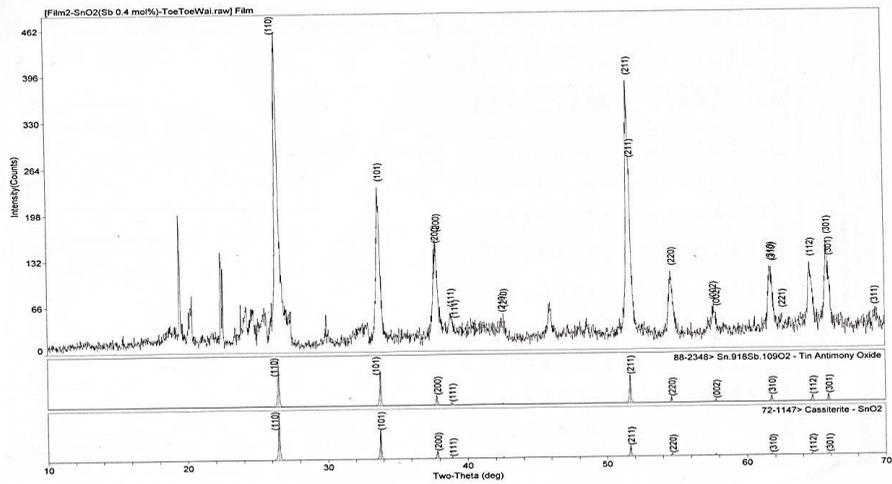
**Figure 1:** (b) XRD patterns obtained for Sb(4 mol% SnO<sub>2</sub>)
