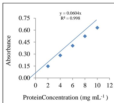
**Figure 3** Calibration curve for standard protein solution
