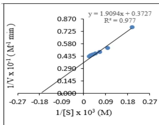
**Figure 9** Lineweaver-Burk plot of  $1/V$  vs.  $1/[S]$  used for graphic evaluation  $V_{max}$  and  $K_m$  for crude peroxidase
