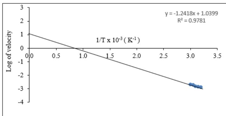
**Figure 6** Plot of log of velocity as a function of 1/T for peroxidase
