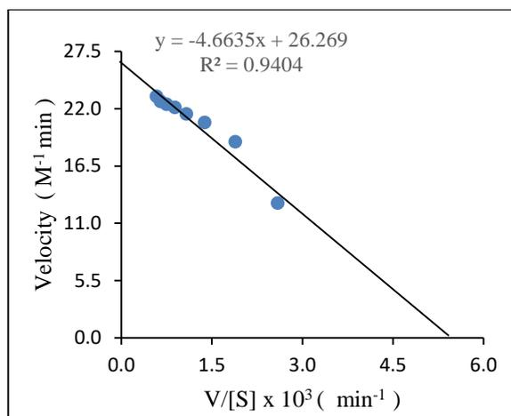
**Figure 10** Eadie-Hofstee plot of  $V$  vs.  $V/[S]$  used for graphic evaluation of  $V_{\max}$  and  $K_m$  for crude peroxidase
