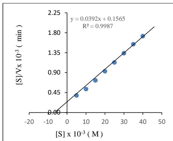
**Figure 11** Hanes-Wilkinson plot of  $[S]/V$  vs.  $[S]$  used for graphic evaluation  $V_{\max}$  and  $K_m$  for crude peroxidase
