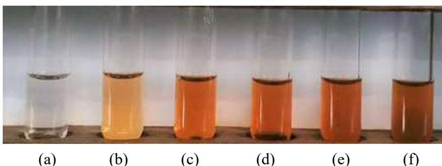
**Figure 1** Mixture of 20 mM guaiacol and 22 mM H<sub>2</sub>O<sub>2</sub> solutions (a) without enzyme (control) and with (b) 11.94 mg mL<sup>-1</sup>, (c) 23.88 mg mL<sup>-1</sup>, (d) 35.82mg mL<sup>-1</sup> (e) 47.76 mg mL<sup>-1</sup> and (f) 59.70 mg mL<sup>-1</sup> enzyme solutions
