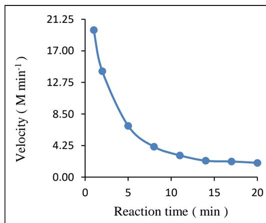
**Figure 7** Plot of velocity of peroxidase-catalyzed reaction as a function of reaction time
