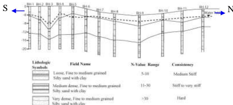
**Figure 12** Idealized cross-section of subsurface soil layers on borehole data
