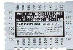
**Figure 6:** Wet Film Thickness Comb
