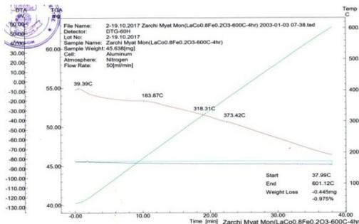
**Figure 7:** TG-DTA thermogram for the  $\text{LaCo}_{0.8}\text{Fe}_{0.2}\text{O}_3$  calcined at  $600\text{ }^\circ\text{C}$
