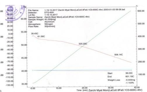
**Figure 8:** TG-DTA thermogram for the  $\text{LaCo}_{0.9}\text{Fe}_{0.1}\text{O}_3$  calcined at  $600\text{ }^\circ\text{C}$
