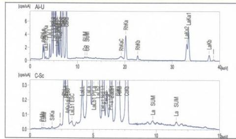
**Figure 19:** EDXRF spectrum of  $\text{LaCo}_{0.9}\text{Fe}_{0.1}\text{O}_3$  nanocrystalline powder
