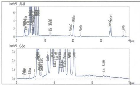
**Figure 18:** EDXRF spectrum of  $\text{LaCo}_{0.8}\text{Fe}_{0.2}\text{O}_3$  nanocrystalline powder
