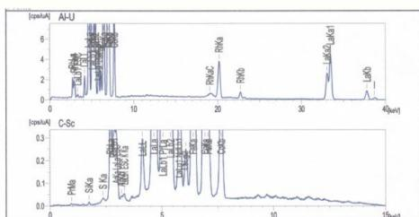
**Figure 16: EDXRF spectrum of  $\text{LaCo}_{0.6}\text{Fe}_{0.4}\text{O}_3$  nanocrystalline powder**
