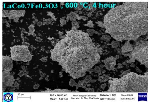
**Figure 22:** SEM micrograph of LaCo<sub>0.7</sub>Fe<sub>0.3</sub>O<sub>3</sub> nanocrystalline powder
