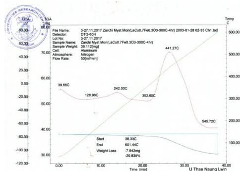
**Figure 2:** TG-DTA thermogram for the  $\text{LaCo}_{0.7}\text{Fe}_{0.3}\text{O}_3$  heated at  $300^\circ\text{C}$
