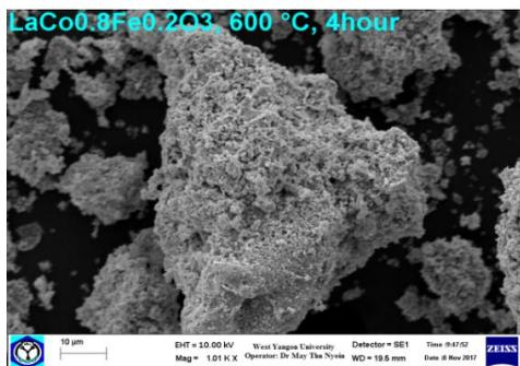
**Figure 23:** SEM micrograph of  $\text{LaCo}_{0.8}\text{Fe}_{0.2}\text{O}_3$  nanocrystalline powder
