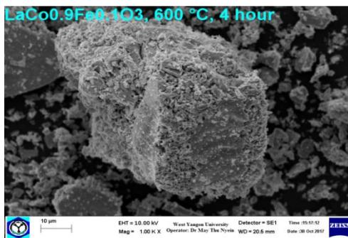
**Figure 24:** SEM micrograph of  $\text{LaCo}_{0.9}\text{Fe}_{0.1}\text{O}_3$  nanocrystalline powder
