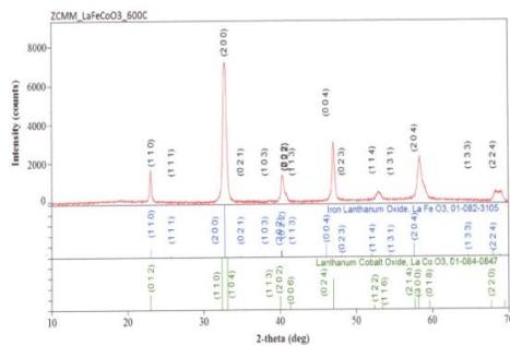
**Figure 10:** XRD patterns of LCFO-SG-I nanocrystalline powder calcined at 600 °C
