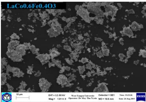
**Figure 21:** SEM micrograph of LaCo<sub>0.6</sub>Fe<sub>0.4</sub>O<sub>3</sub> nanocrystalline powder
