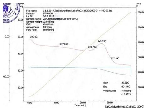
**Figure 1:** TG-DTA thermogram for the  $\text{LaCo}_{0.6}\text{Fe}_{0.4}\text{O}_3$  heated at  $300^\circ\text{C}$
