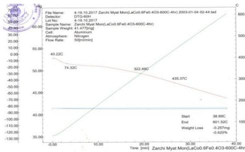
**Figure 5:** TG-DTA thermogram for the  $\text{LaCo}_{0.6}\text{Fe}_{0.4}\text{O}_3$  calcined at  $600\text{ }^\circ\text{C}$
