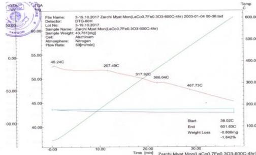
**Figure 6:** TG-DTA thermogram for the  $\text{LaCo}_{0.7}\text{Fe}_{0.3}\text{O}_3$  calcined at  $600\text{ }^\circ\text{C}$
