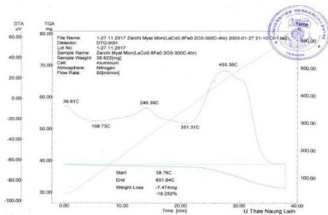
**Figure 3:** TG-DTA thermogram for the  $\text{LaCo}_{0.8}\text{Fe}_{0.2}\text{O}_3$  heated at  $300\text{ }^\circ\text{C}$
