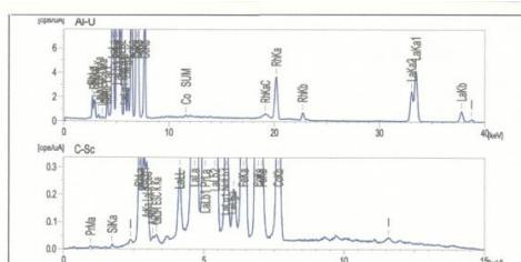
**Figure 17: EDXRF spectrum of  $\text{LaCo}_{0.7}\text{Fe}_{0.3}\text{O}_3$  nanocrystalline powder**
