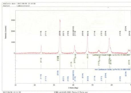
**Figure 9:** XRD patterns of LCFO-SG-I nanocrystalline powders calcined at 500 °C
