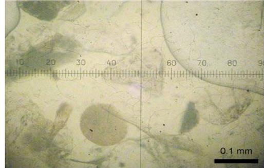
**Figure 13** Photomicrograph showing yellowish colored, rounded phosphate pellet (under PPL) (Sp. 77)
