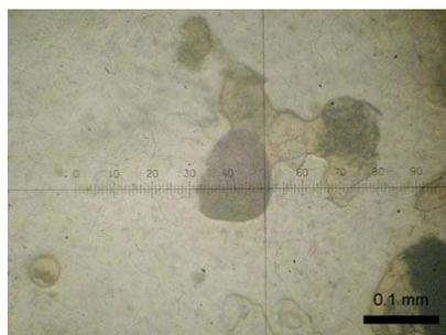
**Figure 2** Photomicrograph showing glauconite grain with minute flakes (under PPL) (Sp. 63).
