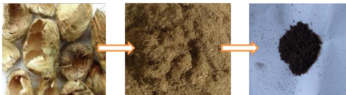
**Figure 2** Conversion of Areca nut Husk biomass into Biochar
