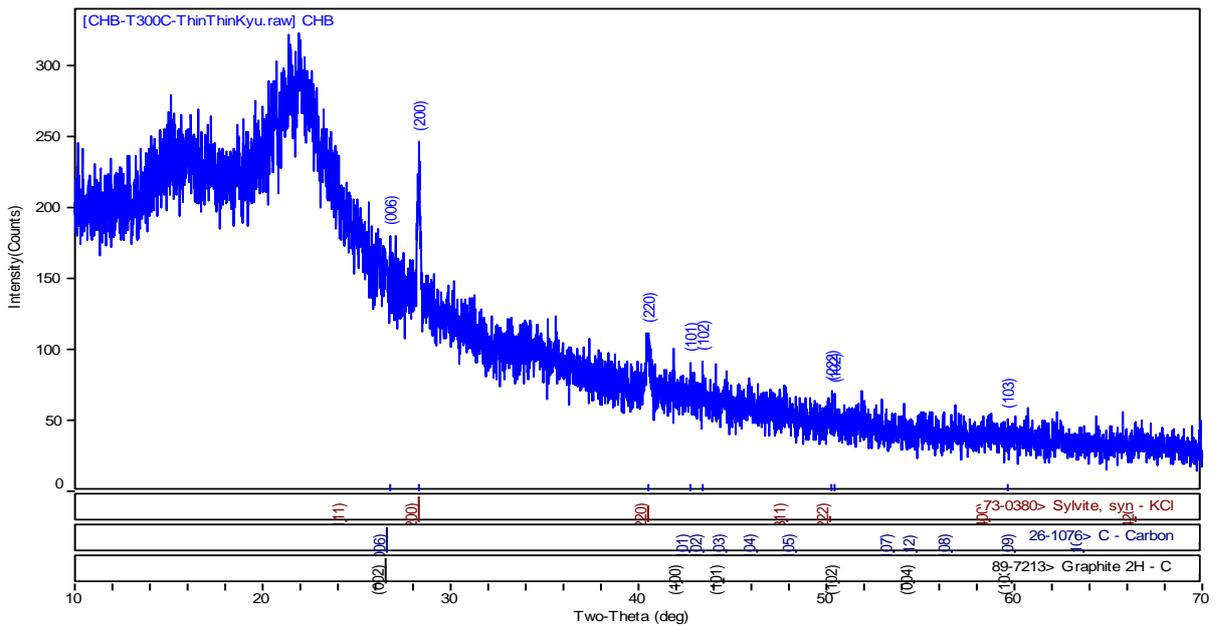
Figure 3 XRD analysis of Coconut Husk Biochar
