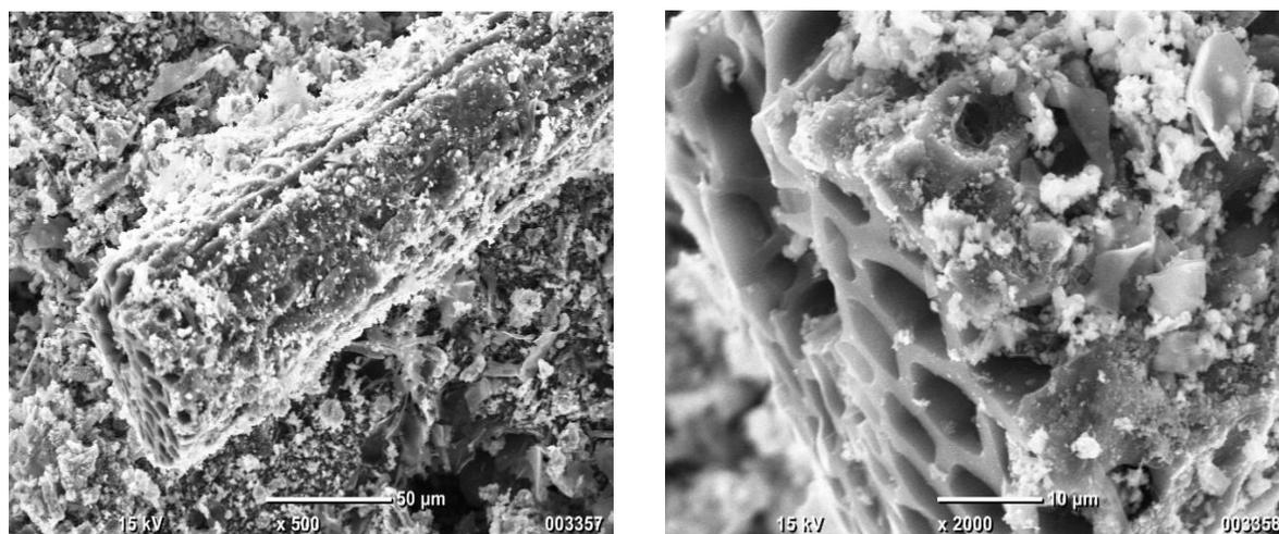
**Figure 8** SEM image of Areca Husk Biochar at (a) 500 X and (b) 2000X magnification
