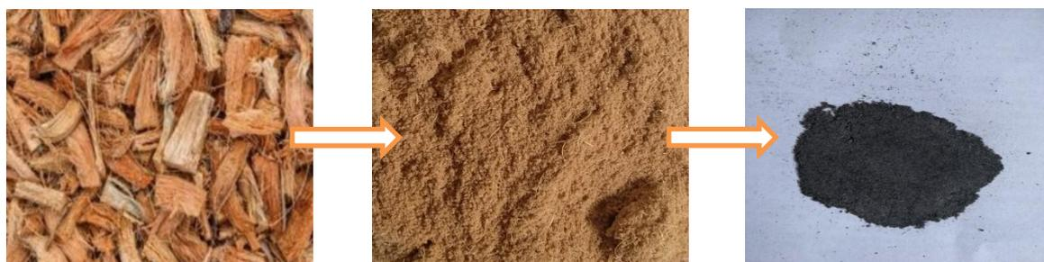
**Figure 1** Conversion of Coconut Husk biomass into Biochar
