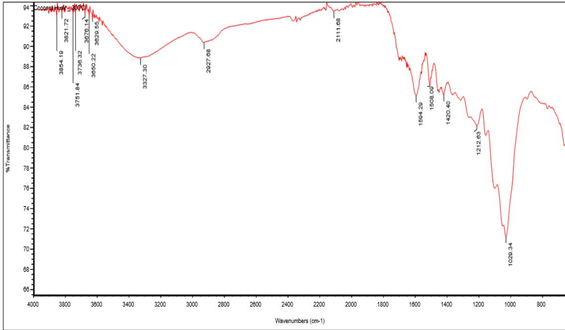
Figure 5 FTIR spectra of Coconut Husk Biochar
