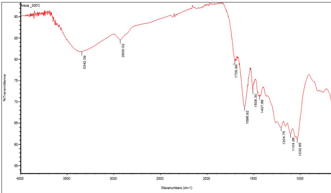
Figure 6 FTIR spectra of Areca nut Husk Biochar
