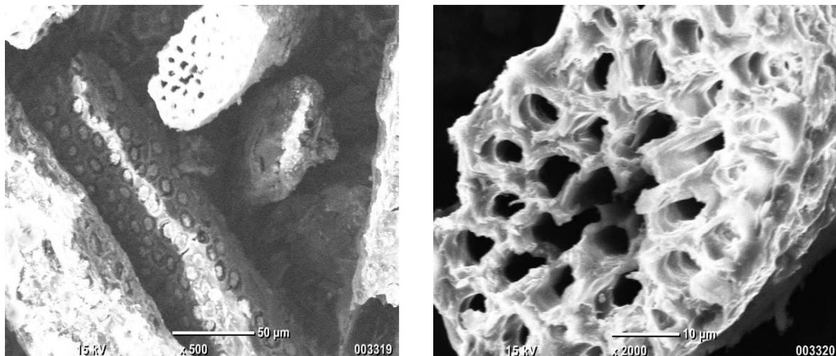
**Figure 7** SEM image of Coconut Husk Biochar at (a) 500X and (b) 2000X magnification
