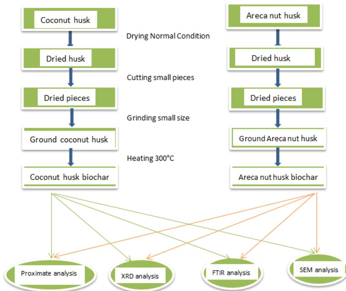
**Figure 3** The flow diagram of the sample preparation of two biochar
