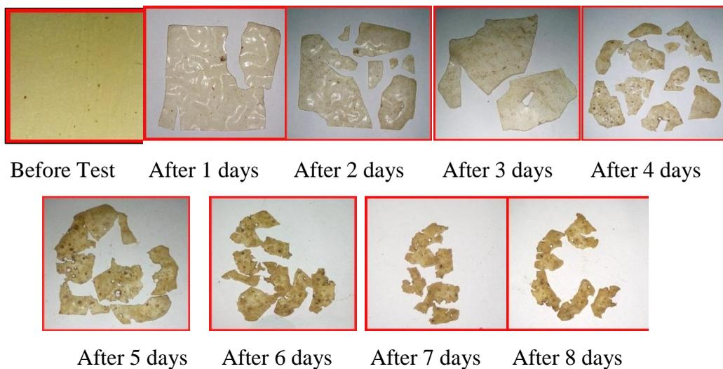
**Figure 8:** Physical appearance changes of chitosan-calcium-alginate composite membrane buried in sandy soil for 8 days
