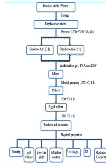
Figure 2. schematic representation of bamboo ash ceramic
