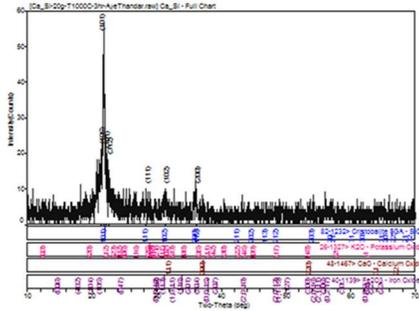
**Figure 3(a).** The XRD pattern of bamboo ash at 1000 °C for 3 h
