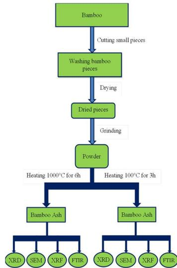
Figure 1. Block diagram of bamboo ash preparation
