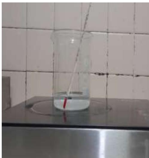
**Figure 4(a).** The etching photograph of CR-39 detector
